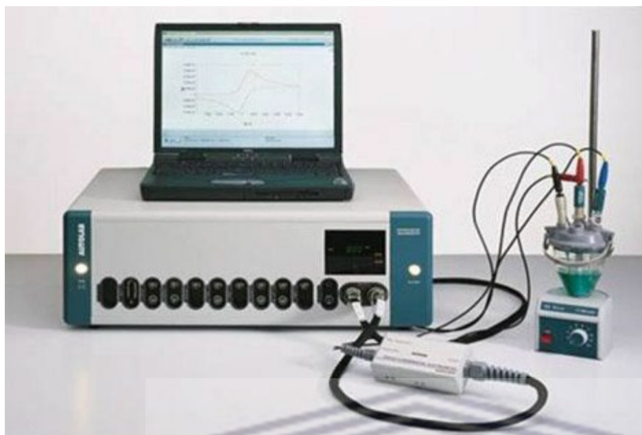
Figure 3. 6: An electrochemical working station showing autolab (galvanostat) and the three Electrodes electrochemical cell assembly [25]
