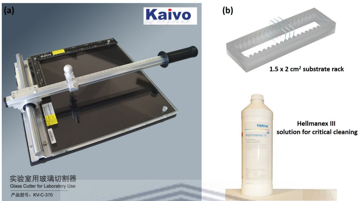
Fig. 2.5: (a) Glass cutter (b) substrate rack and Hellmanex III solution used for sample cleaning
