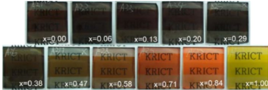
Fig. 1. 11: Degradation of MAPbI 3 thin films, demonstrated by a change in colour from dark brown to yellow, with progressive decrease in the halide concentration [1.39]
