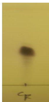
Figure 4.5 TLC silica gel of SC-VII-5 (C1), solvent system silica gel plate; solvent system DCM:MeOH (9.5:05).
