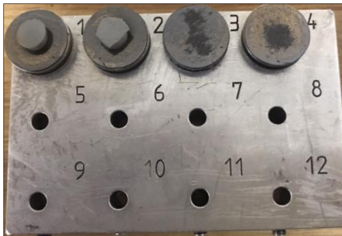
Figure 17. Specimens sputter coated with gold/palladium.
