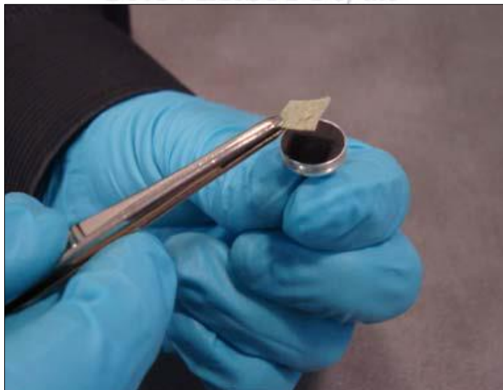
Figure 13. Specimen attached to the stud using carbon adhesive tape.
