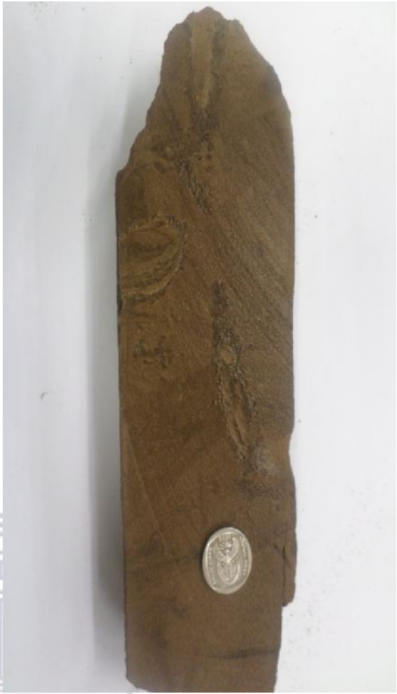
Figure 40: Cylindrical horizontal laminated facies: a. massive or thinly laminated, b. with Ophiomorpha
