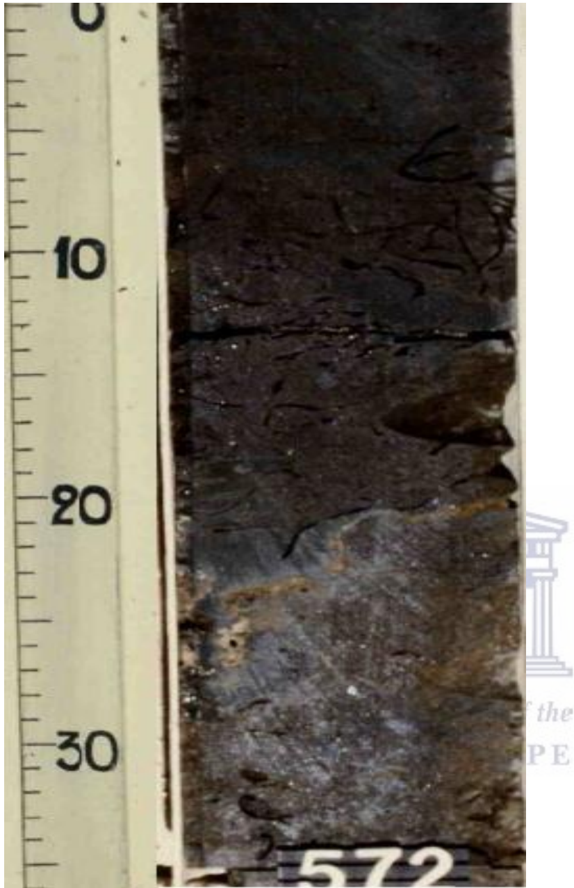
Figure 53: Silty bioclastic packstone (note hardground at 571.80m).
