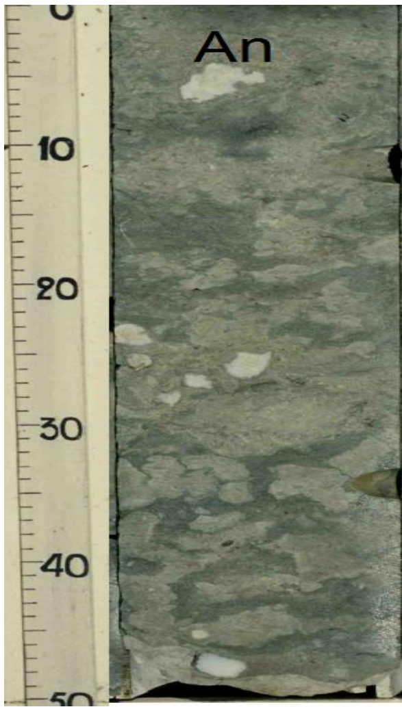
Figure 36: Dolomitic siltstone with anhydrite nodules
