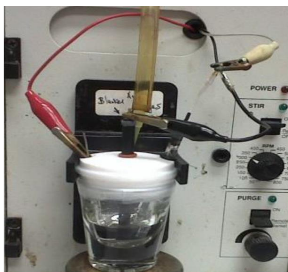
Figure 2.2: A three-way electrode electrochemical workstation for performing characterization of CV, SWV and EIS.
