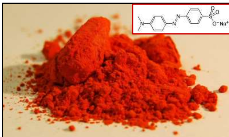
Figure 1: Methyl orange and its structural formula with molecular formula inset
