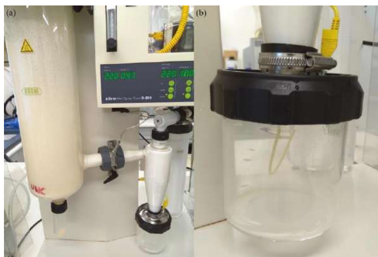
Figure 6.9: Picture showing the lack of powder collection in the collection vessel and complete covering of the drying chamber and cyclone glass with clear distinct separation of the individual feed preparation constituents, as obtained with T14 (Used with permission from the ARC).
