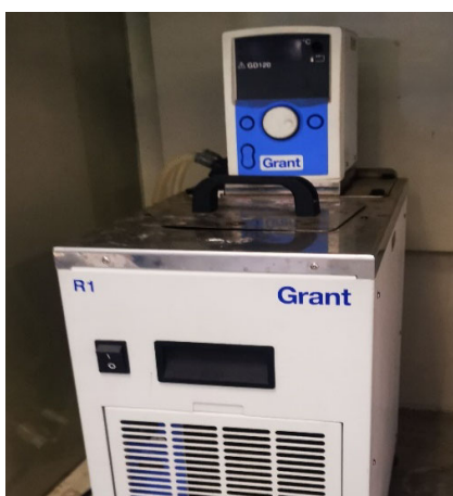
Figure 3.2: Grant R1 thermostatic water bath
