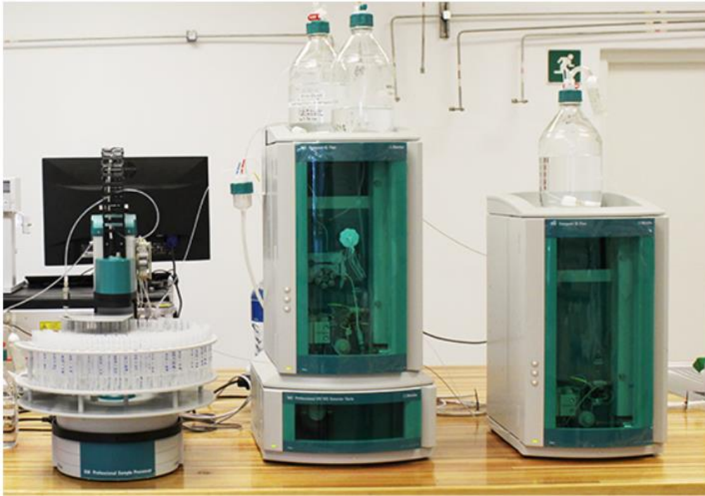
Figure 4.7: Ion chromatography instrument at the BIOGRIP Node for Soil and Water Analysis.
