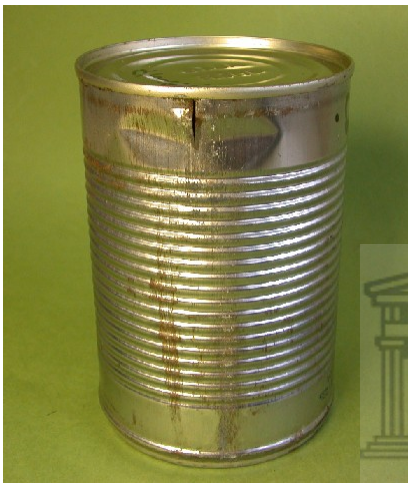
Figure 2-5: A split flange that occurs immediately after the cans are seamed. [2.2]
