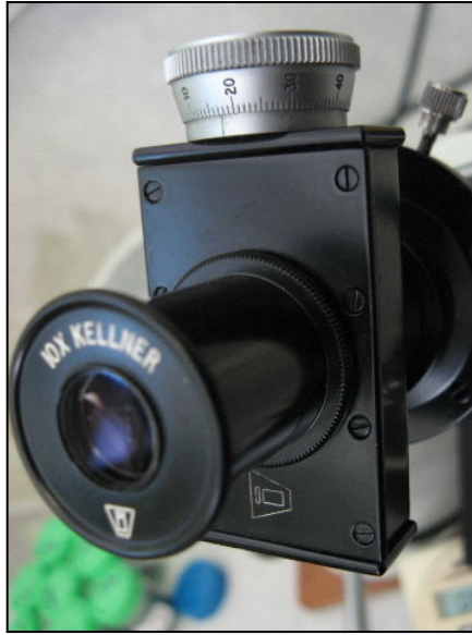
Fig. 11. Filar eyepiece with the filar adjustment knob.
