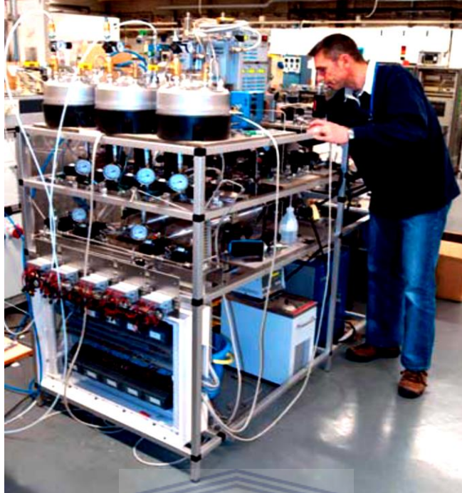
Figure 5.24: Gas handling and temperature control system at JRC-IE [54].
