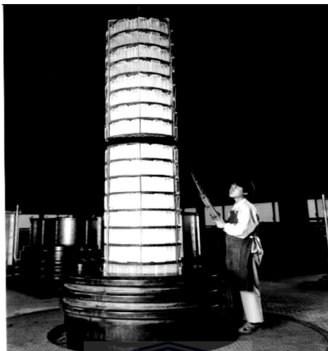
Figure 3.10: Growth of quartz crystals in the world's largest autoclave Japan with >50% production in the world. [27]
