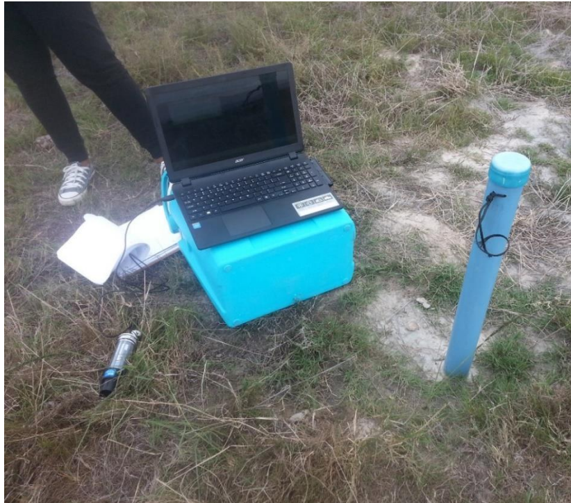
Figure 56: Measuring water level recovery using data loggers
