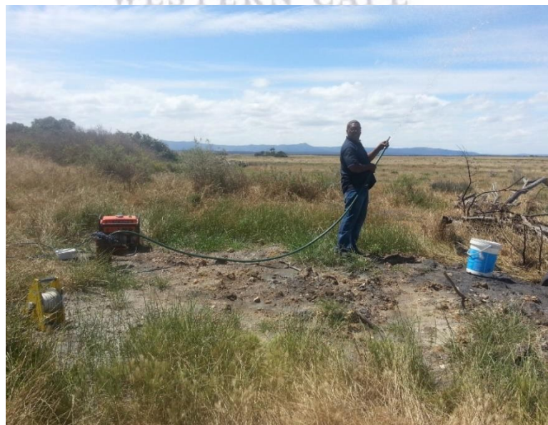
Figure 30: Purging boreholes and piezometers
