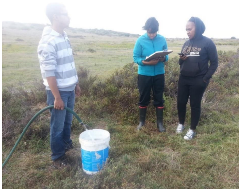
Figure 54: Measuring borehole yields
