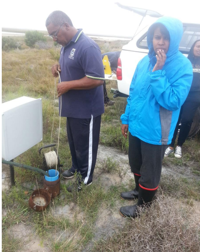
Figure 52: Measuring groundwater levels
