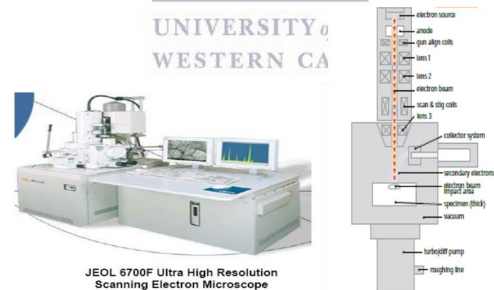
Figure 2-16 Left the JEOL 6700F High Resolution Scanning Electron Microscope adapted from http://www.matter.org.uk/tem/default.htm .
