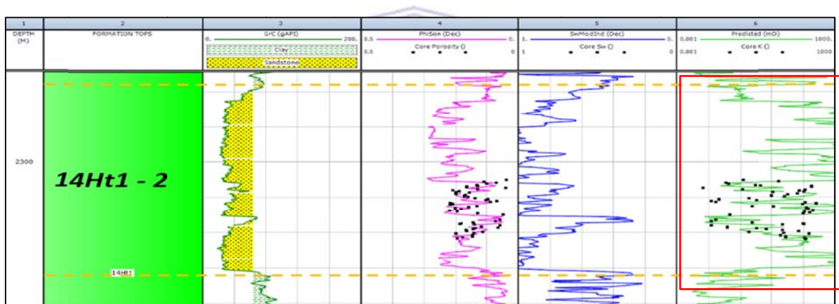
Figure 6.8: Log curves plot displaying predicted permeability with core permeability (track6), well A-F1, reservoir 2.
