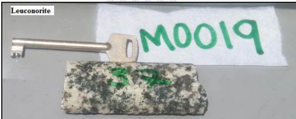
Plate 4.13. A leuconorite at depth 1706.55 m, sample MO019-37, with a coarse grain texture.
