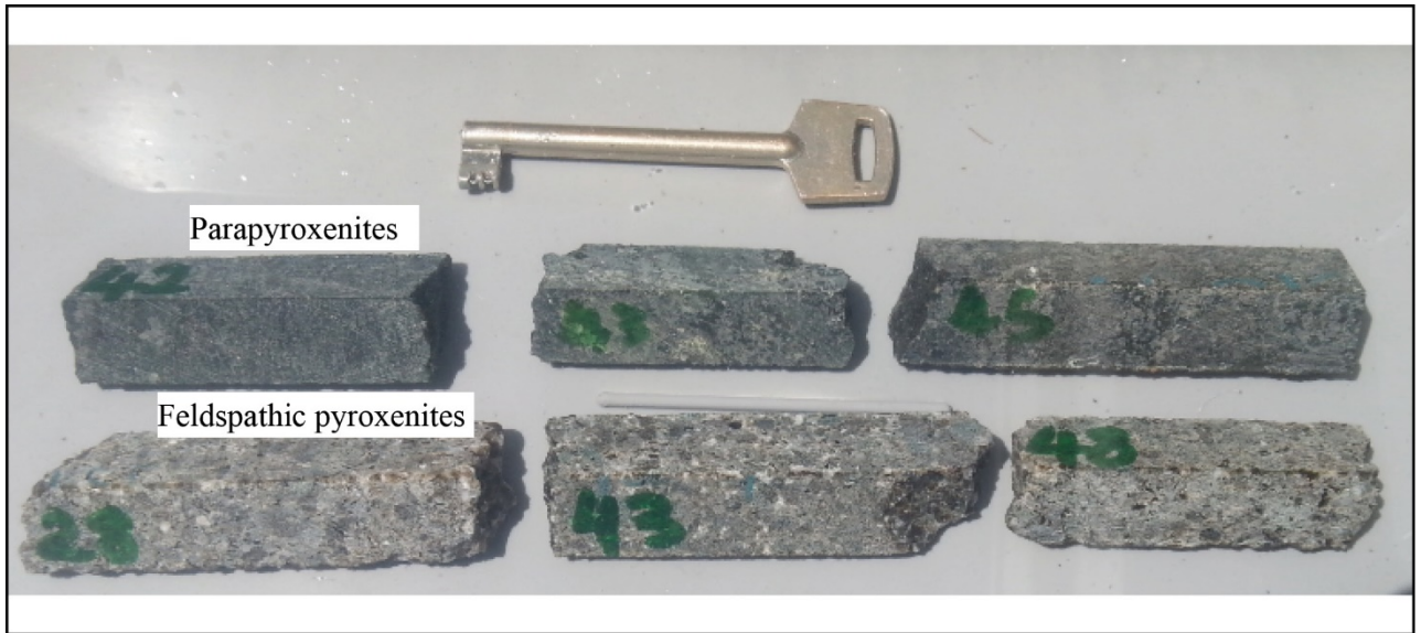
Plate 4.18. The parapyroxenites only found in borehole MO019 and not in MO009, and are compared to the feldspathic pyroxenites which generally present in both the boreholes.
