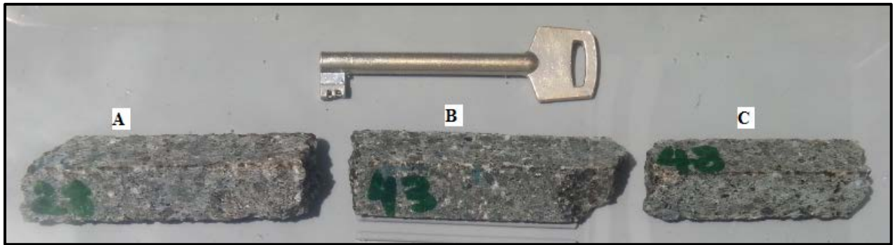
Plate 4.5. A. The feldspathic pyroxenite at a relatively shallower depth of 1,867.26 m (sample MO009-28). B. The feldspathic pyroxenite at relatively middle depth of 1971.03 m (sample MO009-43) white grains of plagioclase are visible. C. The feldspathic pyroxenite at a relatively deeper depth of 1,996.64 m (sample MO009-48).
