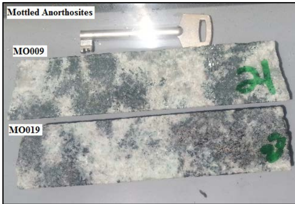
Plate 4.16. The similar lithologies in both boreholes which is the mottled anorthosites and which forms part of the Main Zone.
