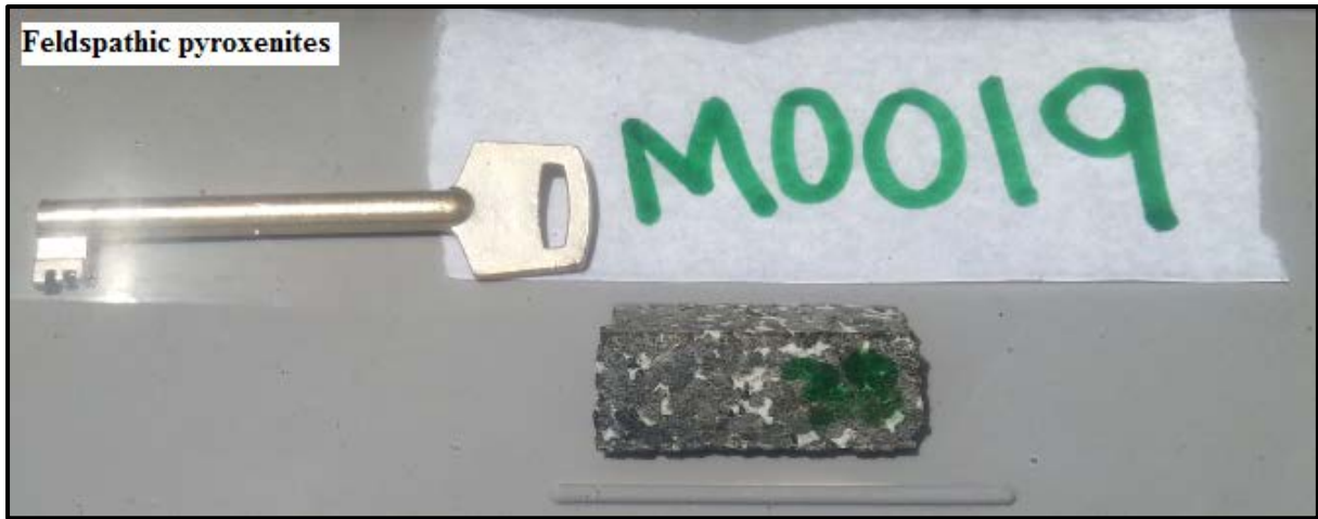
Plate 4.12. A medium- to coarse-grained feldspathic pyroxenite at depth 1717.19 m, sample MO019-38, with visible plagioclase feldspar as white grains.
