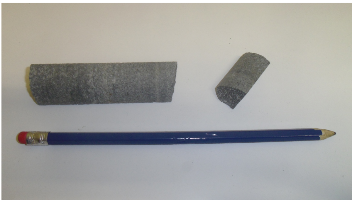
Plate 3.1. A representation of a 50 g cut sample that was crushed and pulverised during sample preparation for XRF laboratory analysis.
