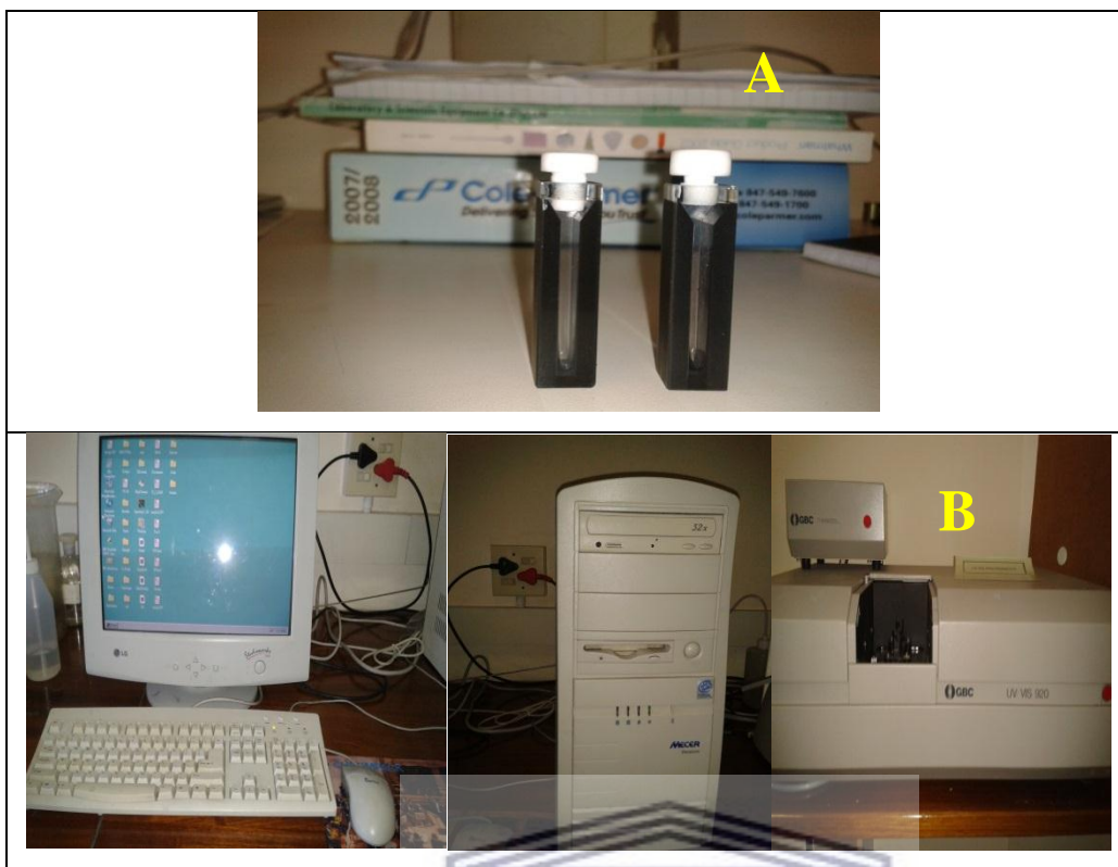
Figure 3.6: GBC UV/VIS 920 spectrometer used for analysis of O.II dye samples.
