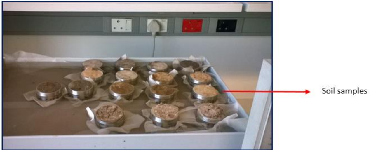
Figure 4.7: Sandbox experiment during pF value 1
