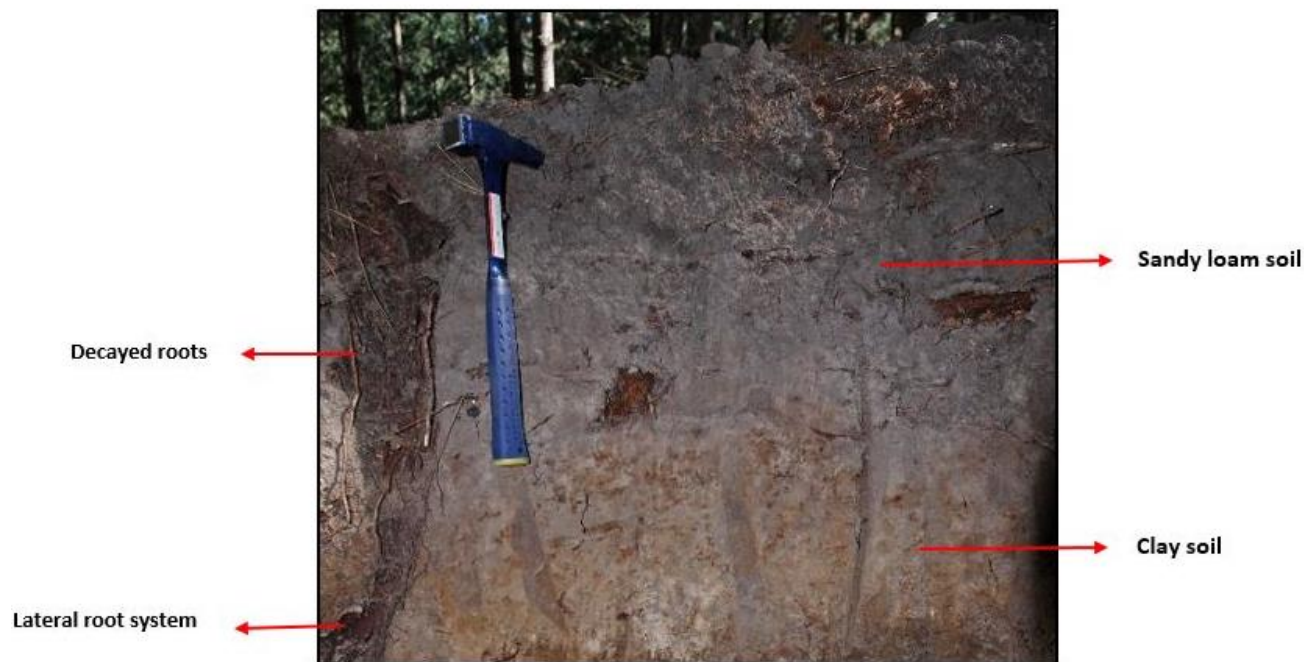
Figure 2.5: Soil profile at the Pinus radiata compartment illustrating the dominant soil types (sandy loam and clay) and root system
