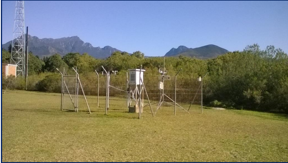
Figure 4.2: An automatic weather station installed in the vicinity of the study site
