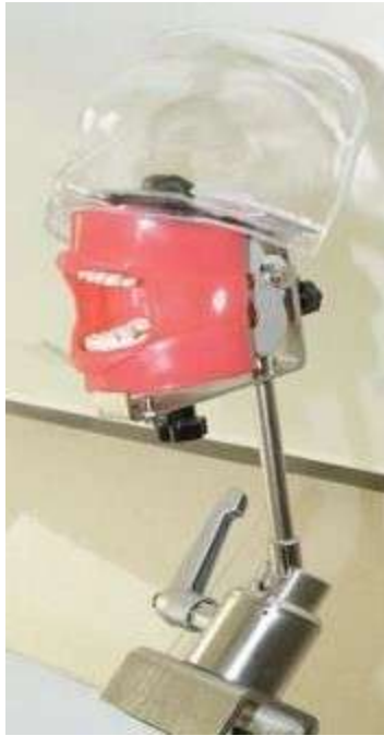
Figure 3.4: Nissim type 2 dental simulator used in the study
