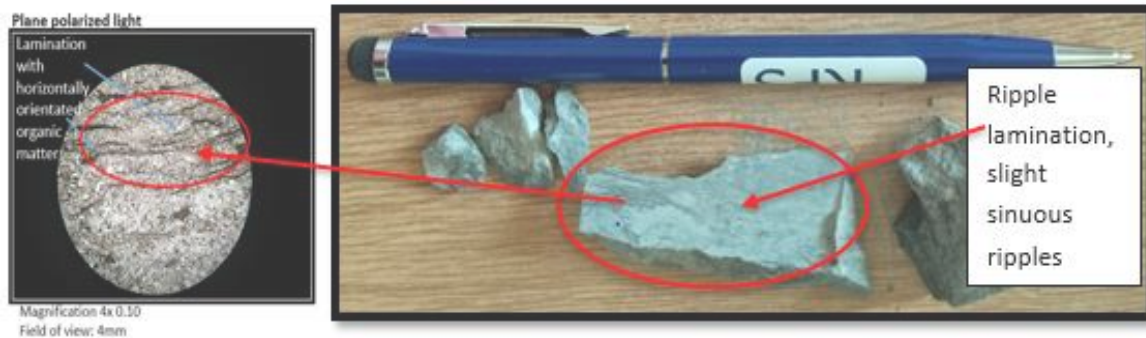
Figure 6. 2: Photomicrograph of sample 7 at 1642 m showing lamination with horizontally orientated organic matter under magnification of 4x 0.10 in the thin section on the left. This corresponds to the shaly sandstone core sample representing facies A on the right.
