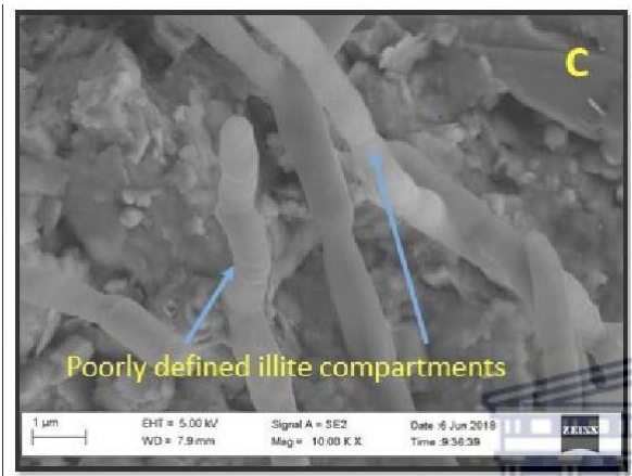
Appendix G5.1: Sample 5 at 3135 m showing well defined quartz crystals in A, randomly orientated illite with platy muscovite in B. A close up of the poorly defined illite compartments is shown in C.
