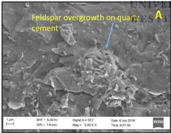
Appendix G5.2: Sample 5.3 at 3135 m showing feldspar overgrowth on quartz cement in A, a close up of the heaped up overgrowth is displayed in B.
