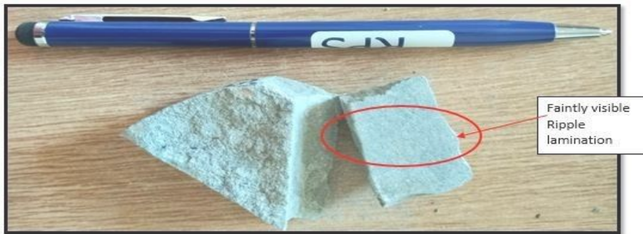
Appendix E1: Core sample 1 of shaly sandstone representing facies B retrieved at 2218 m.
