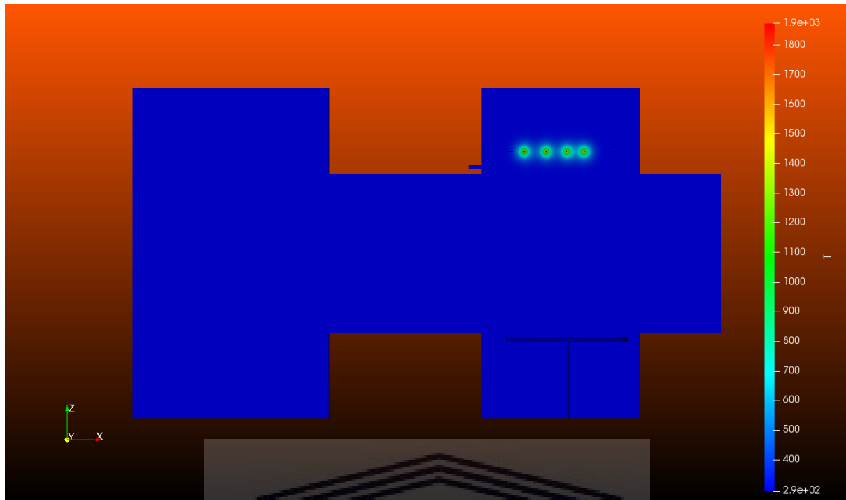
FIGURE 5.8: Convergence temperature for straight wire configuration (K)
