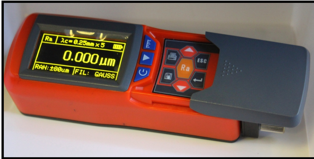
Figure (3.13): Surface roughness machine (Leeb 432 Digital Portable Surface Profile Gauge Precision Roughness Meter with RA RZ range 13 parameters).
