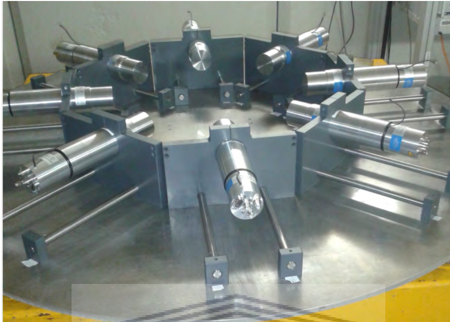
Figure 3.18: An array of 2'' x 2'' LaBr 3 :Ce scintillator detectors commissioned recently at iThemba LABS.
