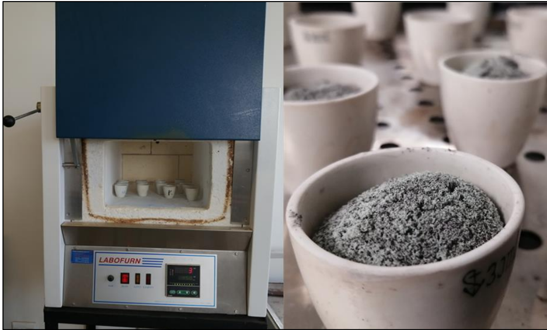
Figure 3. 4: Image showing the muffle furnace used for the sintering as well as the fused end product
