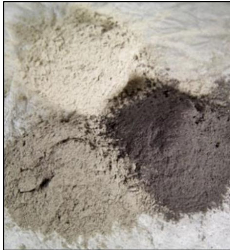
Figure 2. 2: Variations in the colour of coal fly ash (South African Coal Ash Association, 2020)
