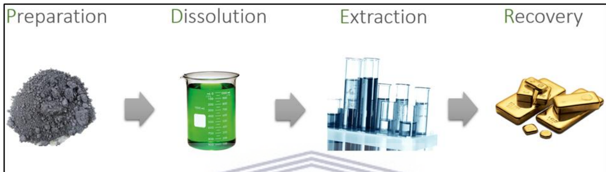
Figure 2. 5: Flow diagram of the general procedure followed in hydrometallurgy for recovering metals from waste material
