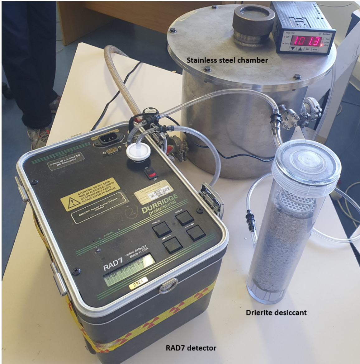
Figure 2.1: The University of the Western Cape(UWC) radon detection setup.
