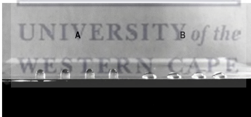
Figure 1-9: The drop collapse test method is used to screen for biosurfactant activity by observing the stability of drops containing biosurfactants on a hydrophobic surface (Clear polyolefin starseal). (A) pure water samples without the presence of biosurfactant. (B) water with the presence of surfactant resulting in the collapsed droplets. Image by Trindade et al. , 2021.
