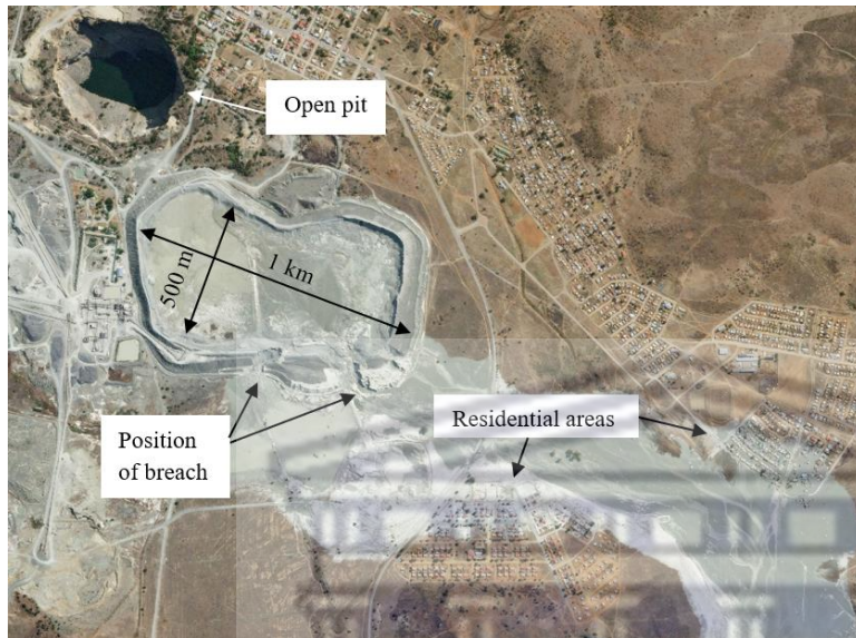
Figure 2.5: Jagersfontein tailings disaster (modified from Planet Team, 2022).
