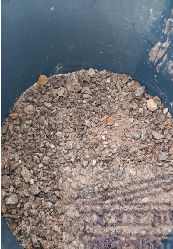
Figure D and E: Course grained aggregate on top of sample and preparation of the sample in predetermined ratios. The soil lab facilities at Cape Peninsula University of Technology was used.
