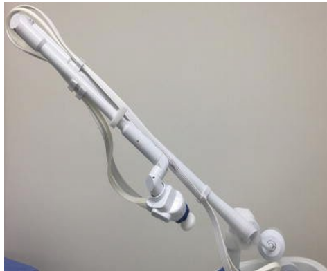
Figure 13: Articulated arm used for indirect contact laser transmission (Coluzzi and Parker, 2017).
