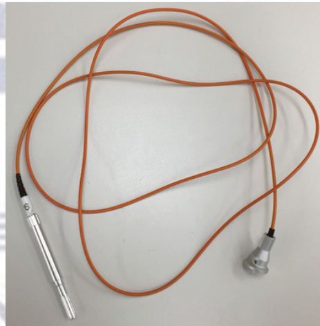
Figure 11: Optical fibre used for direct contact laser transmission (Coluzzi and Parker, 2017).
