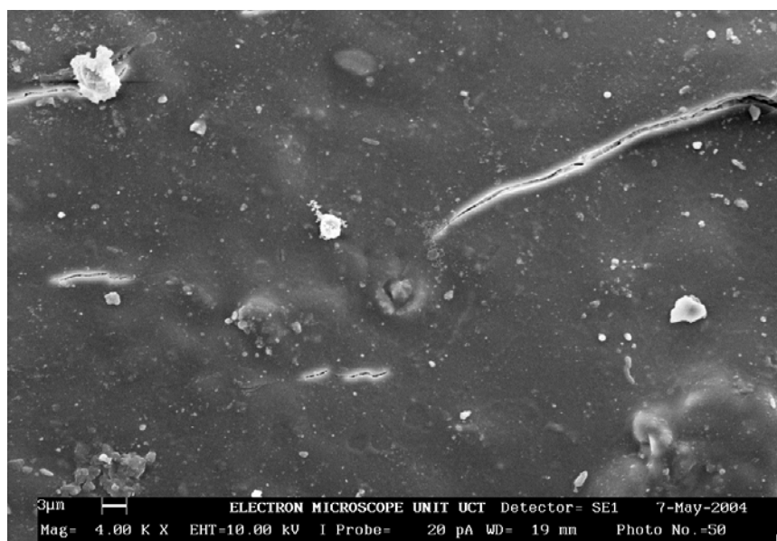
Figure 4.38: SEM micrograph of the surface of CREAFILTER ® S450P impregnated with Nafion ® solution.
