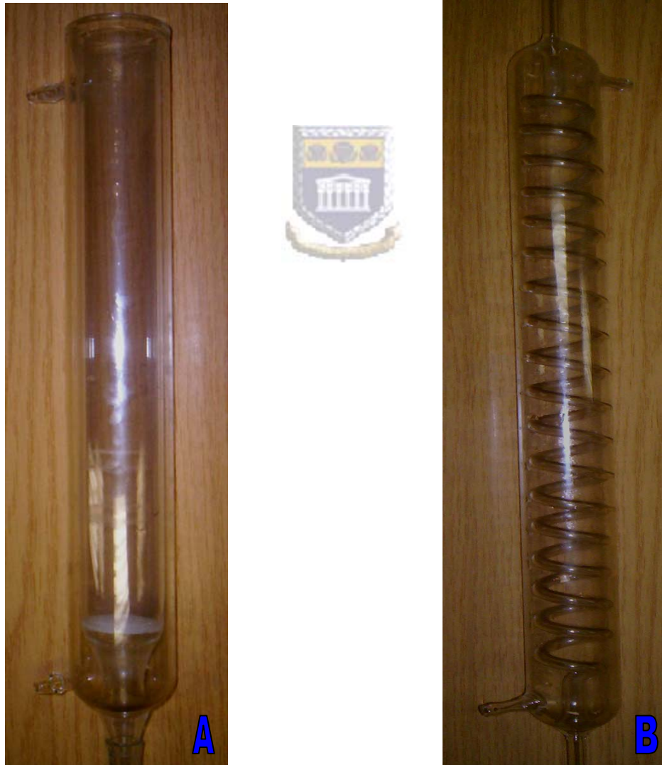
Figure 3.2: Glass condensers: A serves a reservoir for perfusion fluid and is jacketed to keep perfusion fluid at constant temperature. B is used to capture the cardiac output and connects to the reservoir.
