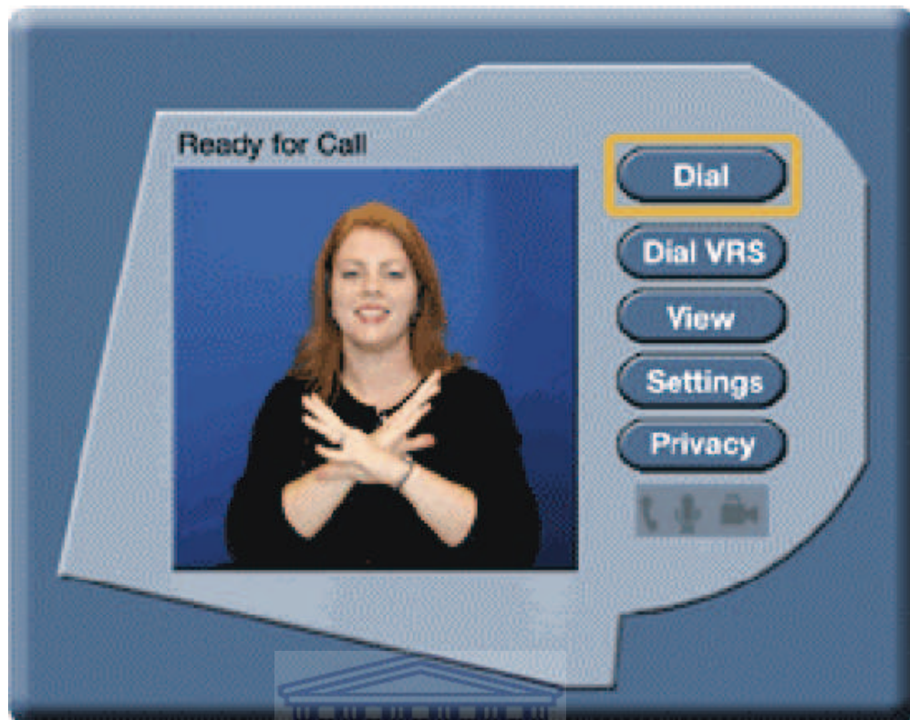
FIGURE 2.3: The user interface of VP-100: The user interface for dial is presented in this figure [19]. A Deaf user selects the menu ‘Dial’ to connect with the relay interpreter. Then the interpreter helps this Deaf user to communicate with a hearing telephone user which whom the Deaf user wants to chat.
