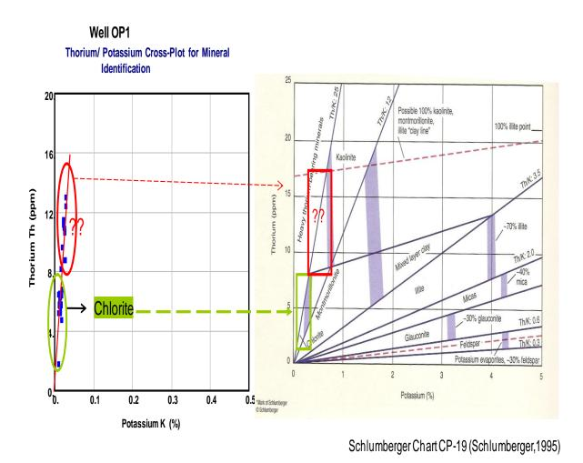
Figure 6.6: Well OP1 potassium/thorium cross plot for identification of clay type
