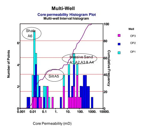
**Figure 5.16**: Permeability histogram for Wells.
