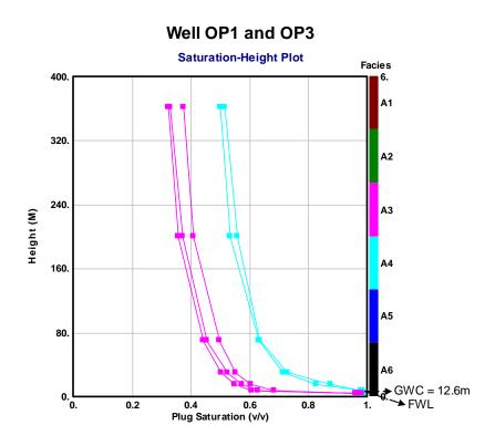
Figure 5.48: Saturation-height function for wells OP1 and OP3
