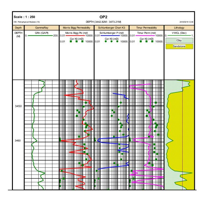
Figure 7.7: Log estimated permeability and overlaid core permeability for well OP2
