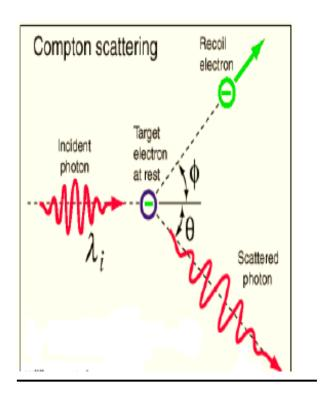
**Figure 2.2**: Compton scattering of gamma rays.
