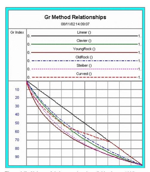
**Figure 6.1b:** Volume of shale correction chart (Schlumberger, 1995)
