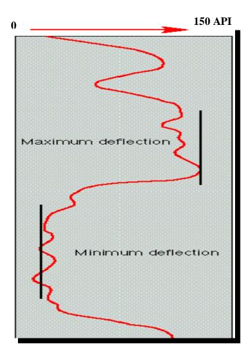
**Figure 2.1**: Diagram of GR log (Modified after Russel, 1944).
