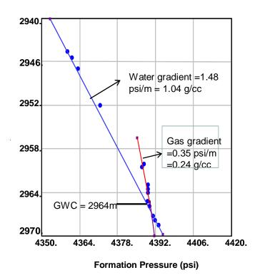
**Figure 8.7**: Well MA2 pressure versus depth plot
