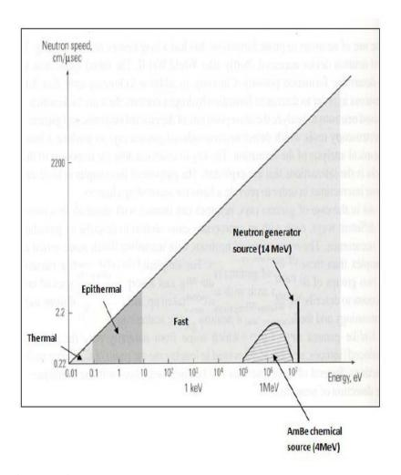
Figure 2.4: Neutron speed versus source (MeV; Ellis & Singer, 1987).
