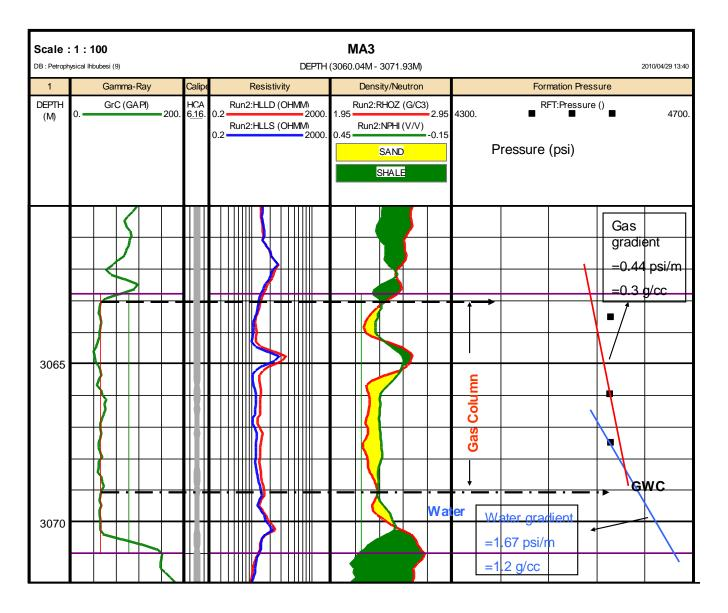
Figure 8.15: Well MA3 comparison of log and pressure data gas water contact
