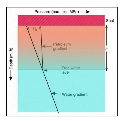
**Figure 3.7**: Pressure versus depth plot.
