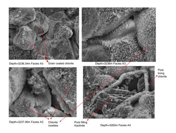
Figure 5.36: Example of Well OP3 SEM analysis result
