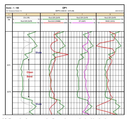
Figure 4.2: Example of gamma-ray log Run at the same depth with other logs.
