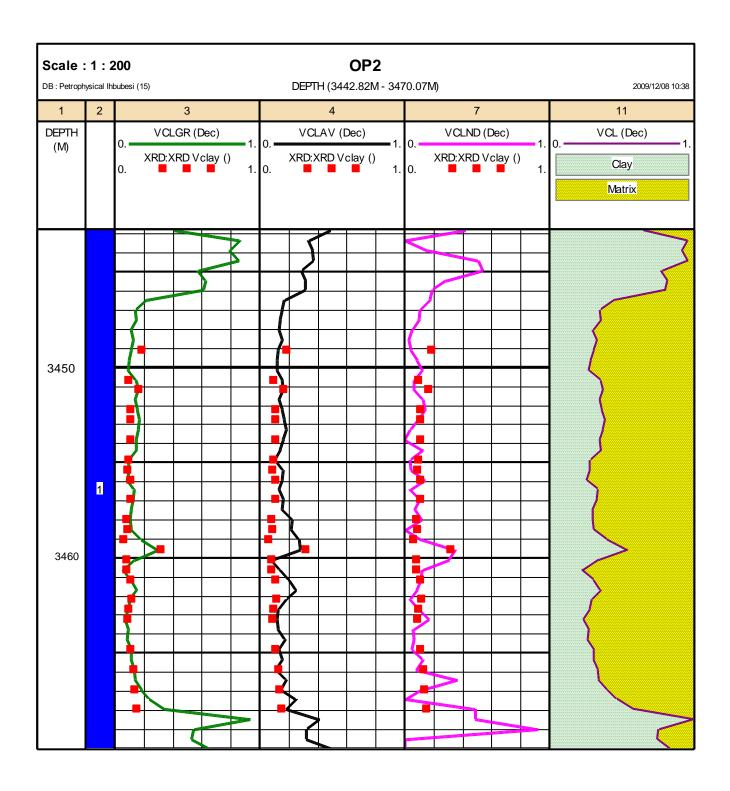
**Figure 6.3**: Log determined volume of clay overlain with XRD volume of clay for well OP2.
