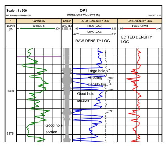
Figure 4.3: Example of density log affected by borehole.
