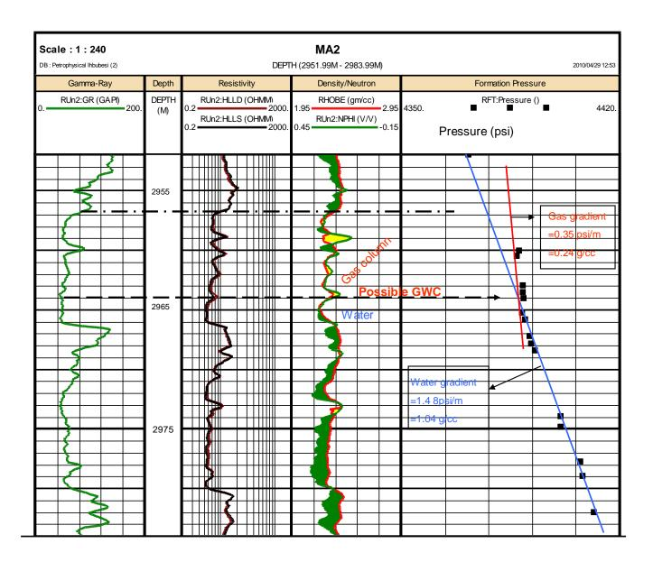
Figure 8.14: Well MA 2 comparison of log and pressure data gas water contact
