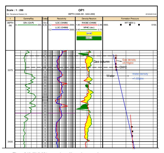
Figure 8.10: Well OP1 comparison of log and pressure data gas water contact
