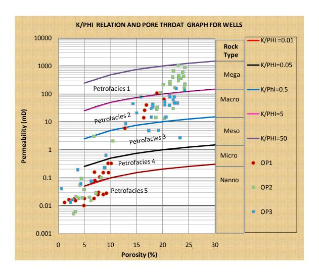
**Figure 7.15e**: Permeability/Porosity Ratio (K/PHI) for all the wells
