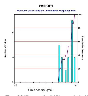
Figure 5.5: Histogram of well OP1 core grain densities.
