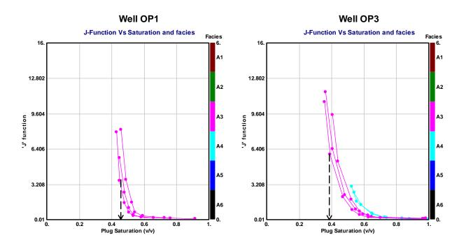
Figure 5.47: J-function curves for well OP1 and OP3
