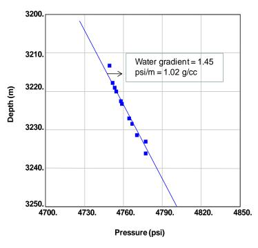
**Figure 8.6**: Well MA1 pressure versus depth plot
