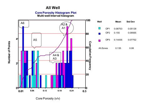
**Figure 5.12a**: Histogram of Porosity distribution for wells.
