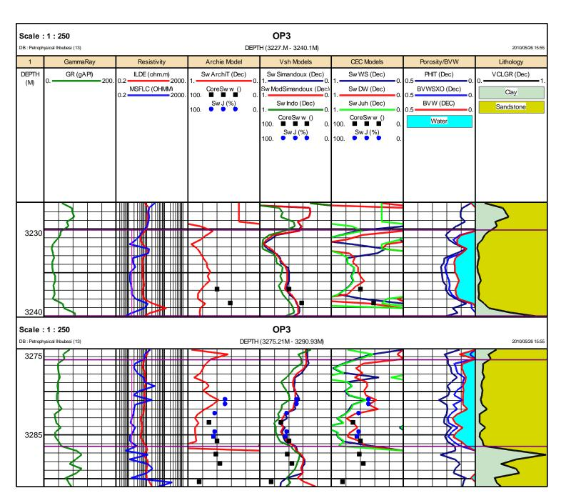
Figure 6.17: Comparison of core and log water saturation models for Well OP3
