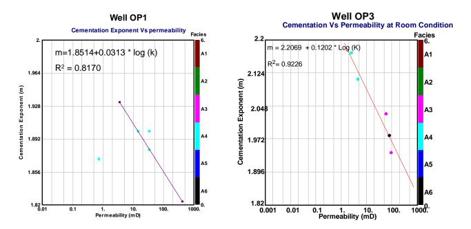
Figure 5.28: Well OP1 and OP3 cementation exponent Vs permeability at room temperature
