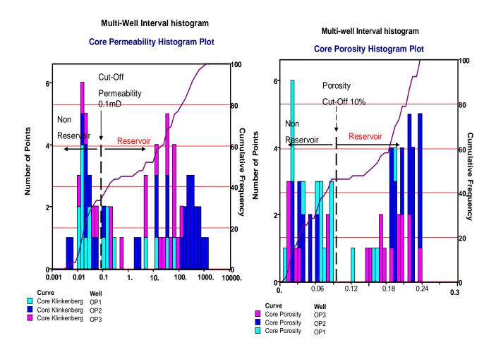
Figure 9.8b: Multi-Well permeability and porosity histogram distributions
