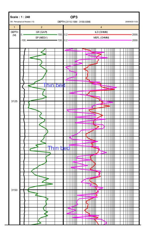
**Figure 4.5**: Thin bed recognition on resistivity logs
