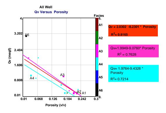
Figure 5.40a: Plot of Qv versus Total and effective porosities for all Well
