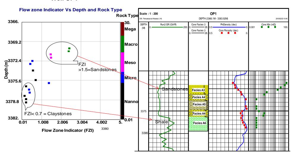
Figure 7.16a: Well OP1 flow zone indicator, rock types and facies plot
