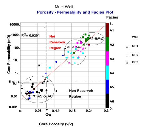
Figure 9.8a: Multi-Well porosity-permeability plot for cut-off determination
