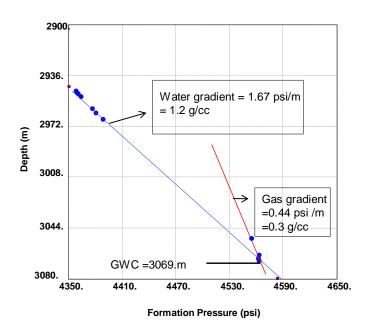
Figure 8.8: Well MA3 pressure versus depth plot
