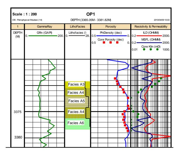
Figure 5.2: Well OP1 showing core facies in track 3.
