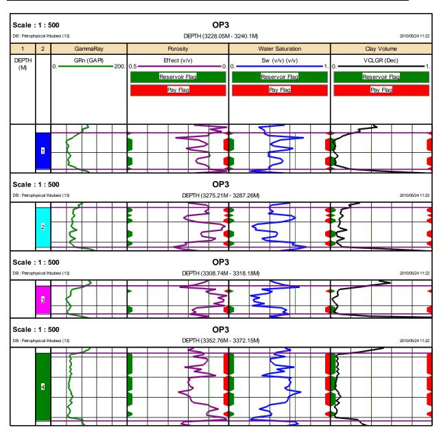
Figure 9.14: Well OP3 graphics of calculated reservoir parameters and flags
