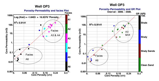
Figure 5.21: Porosity-Permeability and facies GR plot for Well OP3
