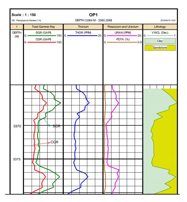
Figure 6.5: Well OP1 spectral gamma ray log
