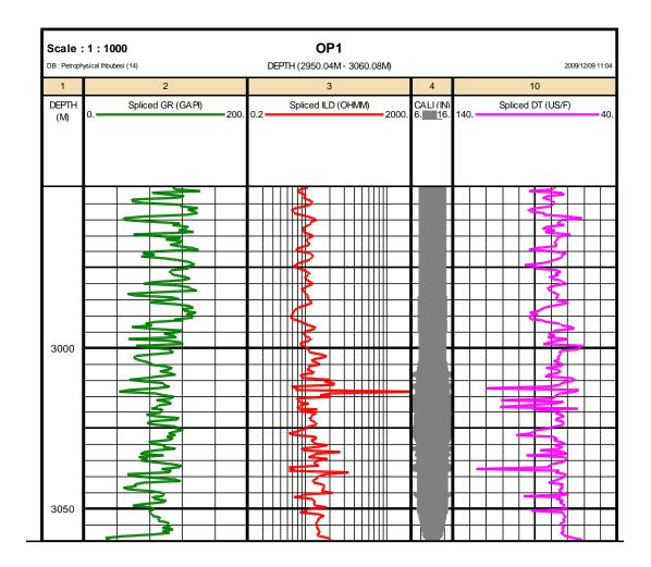
Figure 4.7b: Examples of graphics of spliced curves
