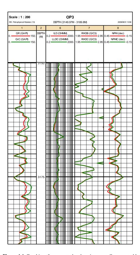
Figure 4.4: Graphics of uncorrected and environmentally corrected logs
