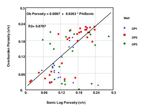
Figure 6.10: Multi-Well overburden porosity versus log porosity
