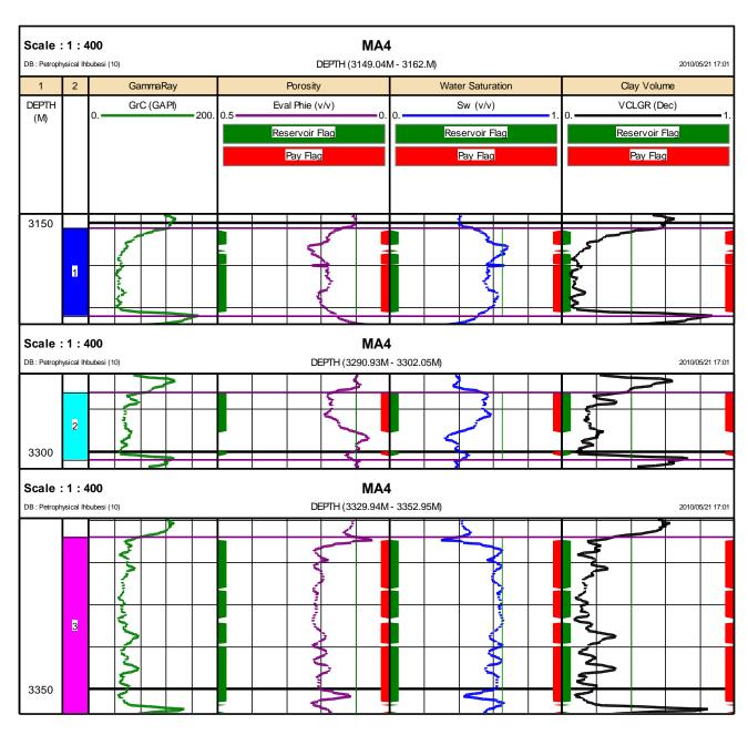
Figure 9.20: Well MA4 graphics of calculated reservoir parameters and flags
