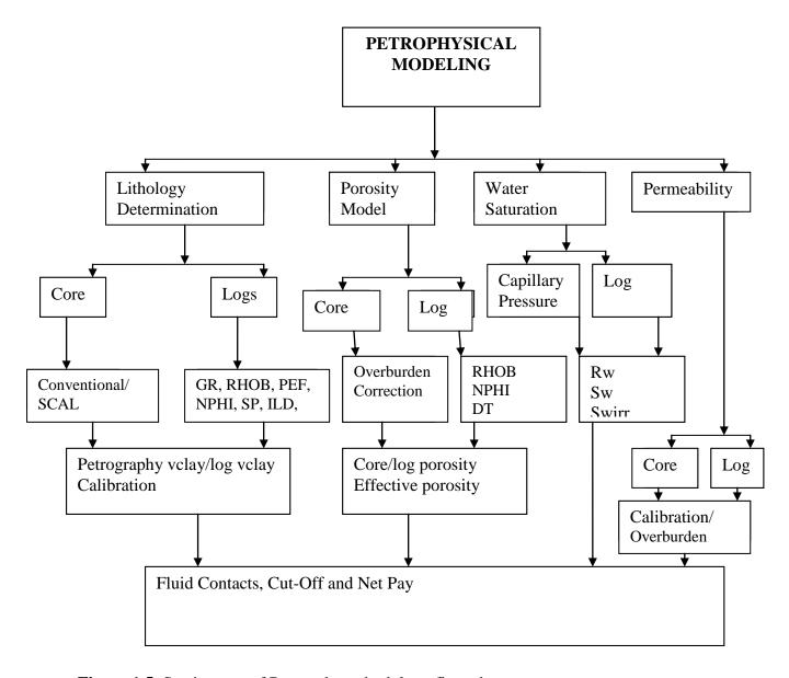
Figure 1.5: Section two of Research methodology flow chart.
