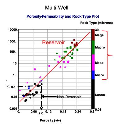
Figure 9.8c: Application of permeability and porosity cut-off to petrofacies
