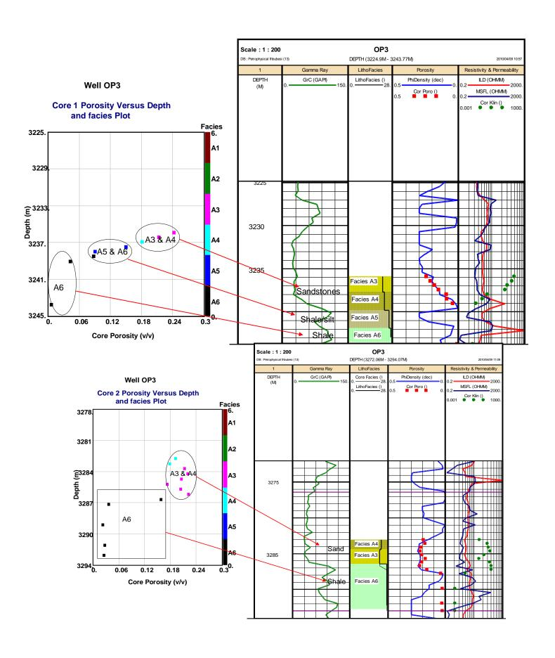
Figure 5.11a: Well OP3 porosity versus depth plot
