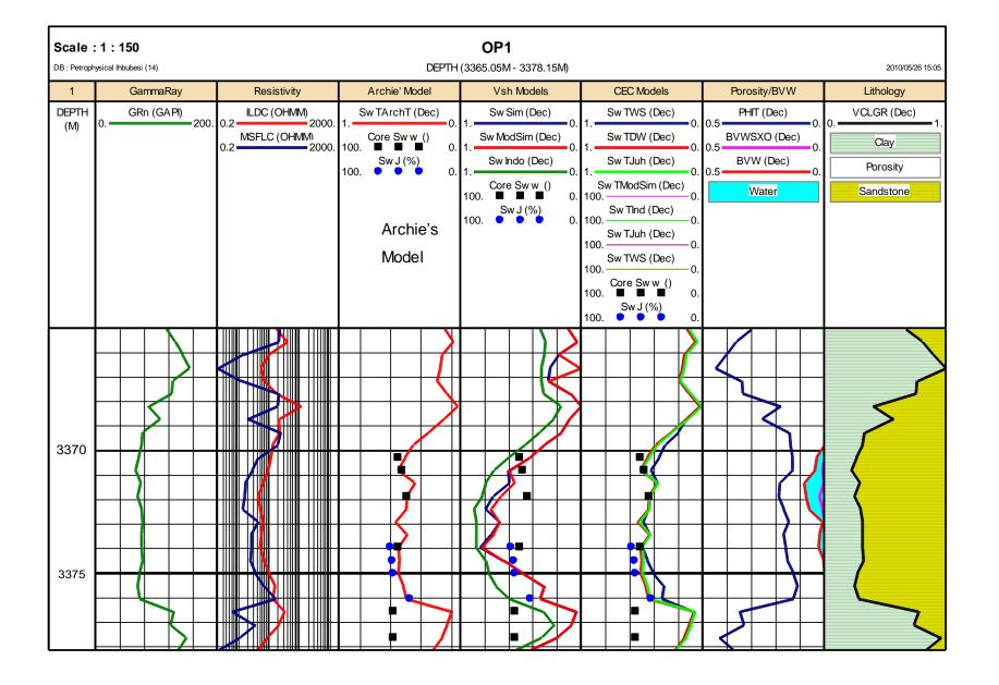
Figure 6.16: Comparison of core and log water saturation models for Well OP1
