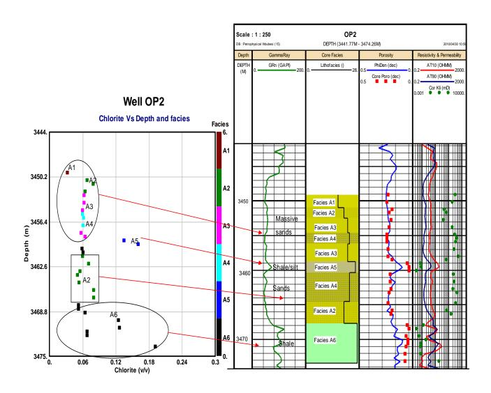
Figure 5.37: Distribution of chlorite for Well OP2
