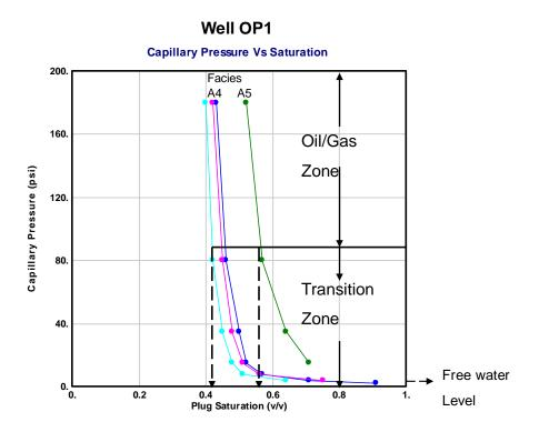
Figure 5.42: Capillary pressure curve for well OP1
