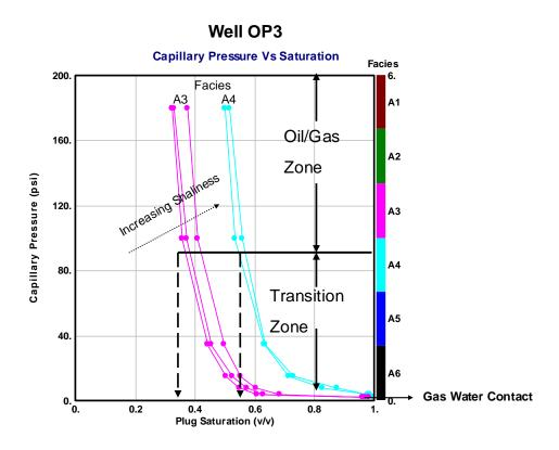
Figure 5.43: Capillary pressure curve for Well OP3
