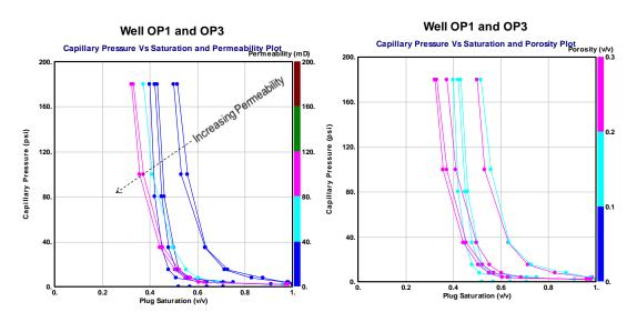
Figure 5.45: Capillary pressure curves with permeability and porosity
