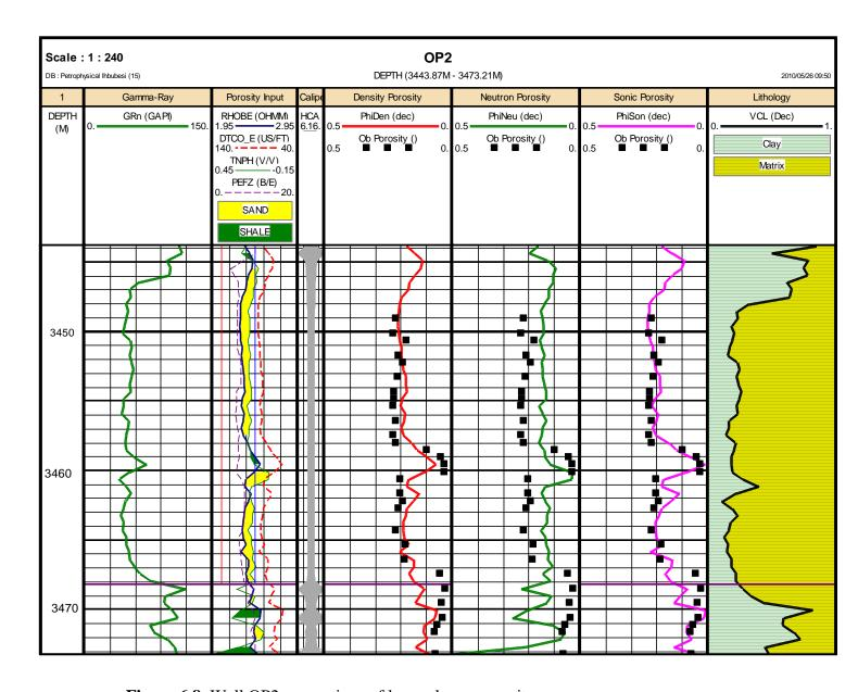
Figure 6.8: Well OP2 comparison of log and core porosity.
