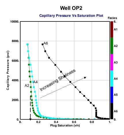
Figure 5.44: Capillary Pressure Curve for Well OP2
