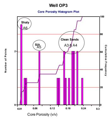
Figure 5.11b: Histogram of well OP3 core porosity distribution.
