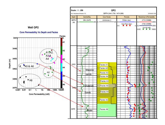
Figure 5.14a: Well OP2 Depth versus permeability plot.
