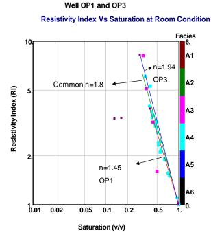
Figure 5.31: Resistivity index versus saturation plots for well OP1 and OP3
