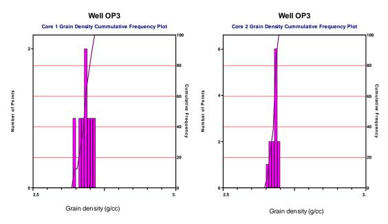
**Figure 5.7**: Well OP3 core grain density cumulative frequency plot.
