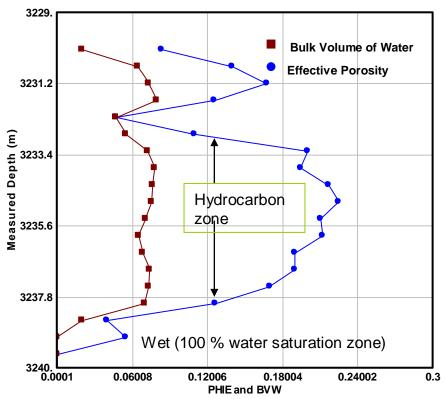
Figure 6.18: Bulk volume of water and effective porosity plot for well OP3
