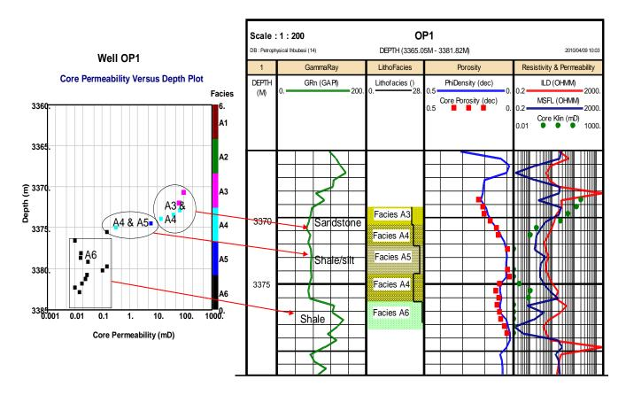
Figure 5.13a: Well OP1 permeability versus depth Plot.
