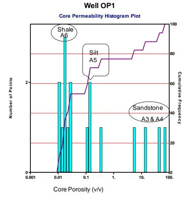
Figure 5.9b: Histogram of porosity distribution for well OP1
