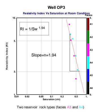
Figure 5.30: Well OP3 resistivity index versus saturation plot
