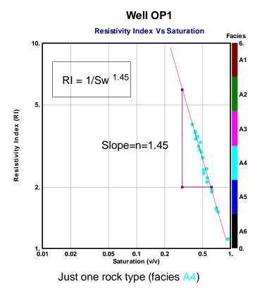
Figure 5.29: Well OP1 resistivity index versus water saturation plot.
