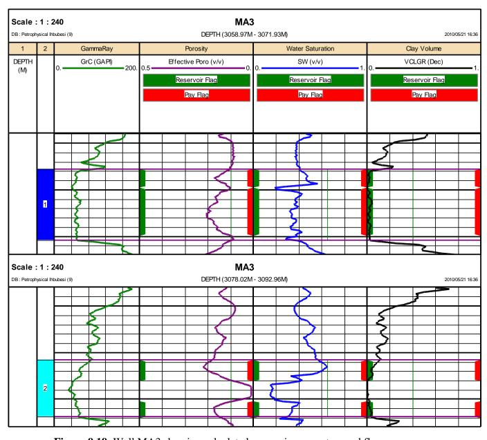
Figure 9.19: Well MA3 showing calculated reservoir parameters and flags
