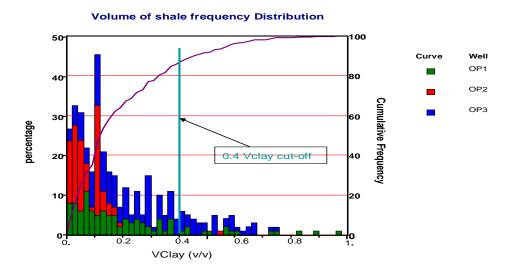
Figure 9.9b: Multi-Well vclay frequency distribution and cut-off point
