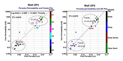
Figure 5.20: Porosity-Permeability and facies and GR plot for well OP2
