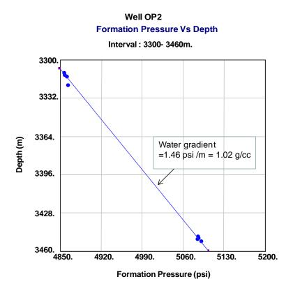
Figure 8.2: Well OP2 pressure versus depth plot
