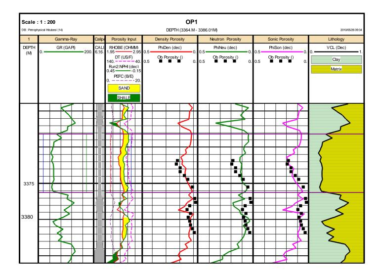
Figure 6.7: Well OP1 comparison of log and core porosity
