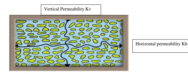
**Figure 3.4**: Directions of measurement of permeability.
