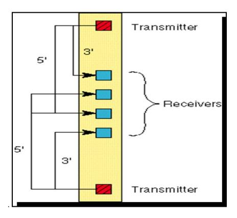
Figure 2.5: The positions of transmitters and receivers in sonic tool.
