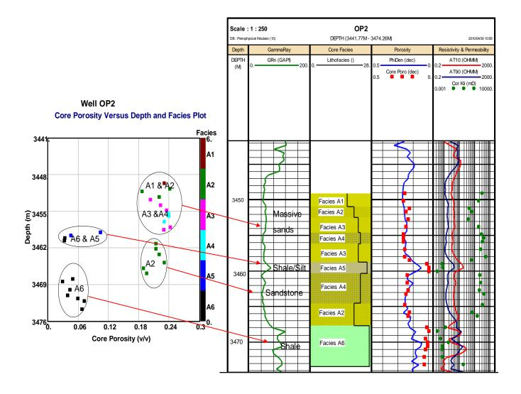
Figure 5.10a: Well OP2 porosity versus depth plot.
