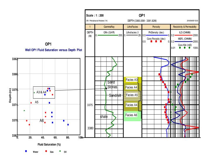
Figure 5.17: Well OP1 fluid saturation versus depth plot.
