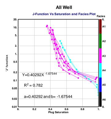
Figure 5.46: Leverett's saturation determination J-function
