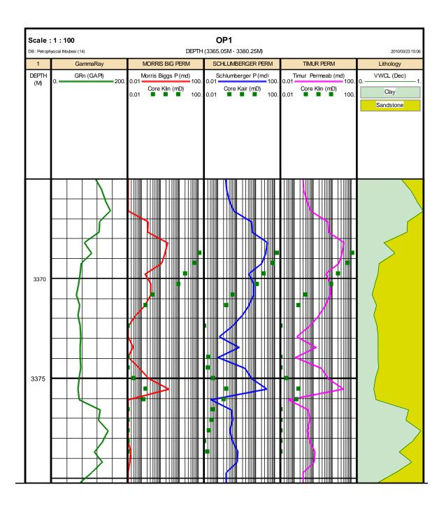
Figure 7.6: Log estimated permeability and overlaid core permeability for well OP1
