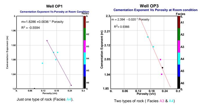
Figure 5.26: Well OP1 and OP3 cementation versus porosity plot at room conditions.
