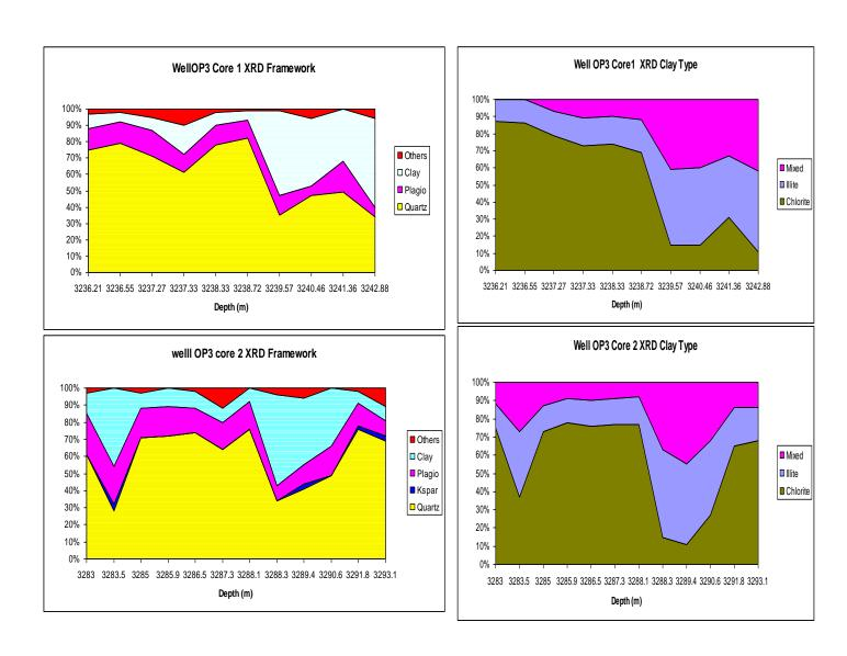
Figure 5.34: Whole rock mineralogy of core 1 and 2 of well OP3
