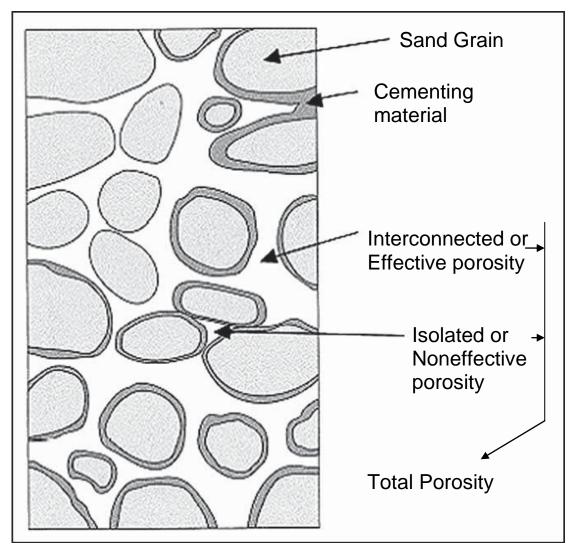
Figure 3.2: Example of effective and total porosity.
