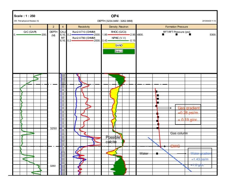
Figure 8.12: Well OP4 Comparison of log and pressure data gas water contact
