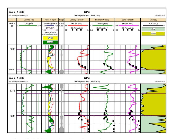
Figure 6.9: Well OP3 comparison of log and core porosity
