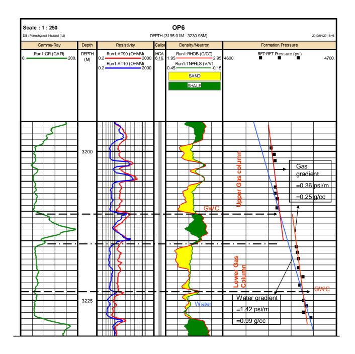
Figure 8.13: Well OP6 Comparison of log and pressure data gas water contact
