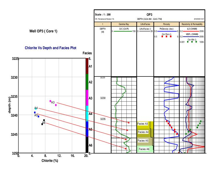
Figure 5.38a: Well OP3 core 1 chlorite distribution
