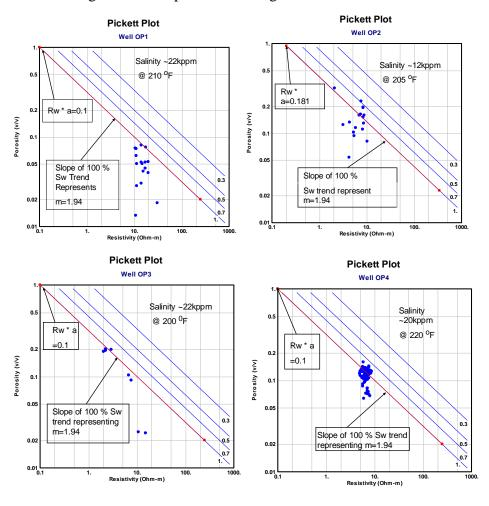
**Figure 6.12**: Pickett Plot for determination of resistivity of water (Rw) for well OP1, OP2, OP3, and OP4 respectively.
