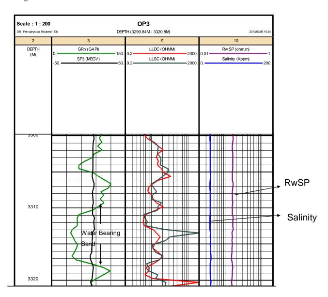
Figure 6.11: Example of resistivity of water from SP method
