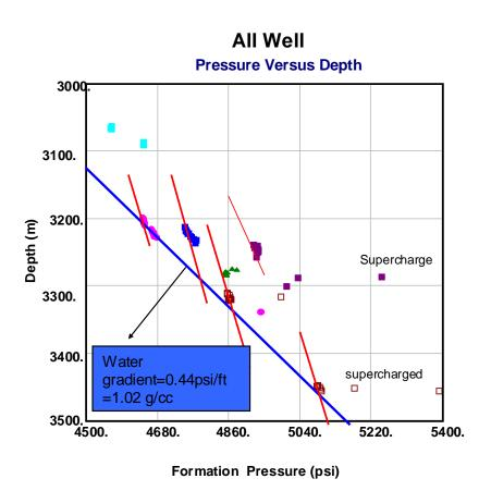
Figure 8.9: Overlaid gas and water gradients in the field
