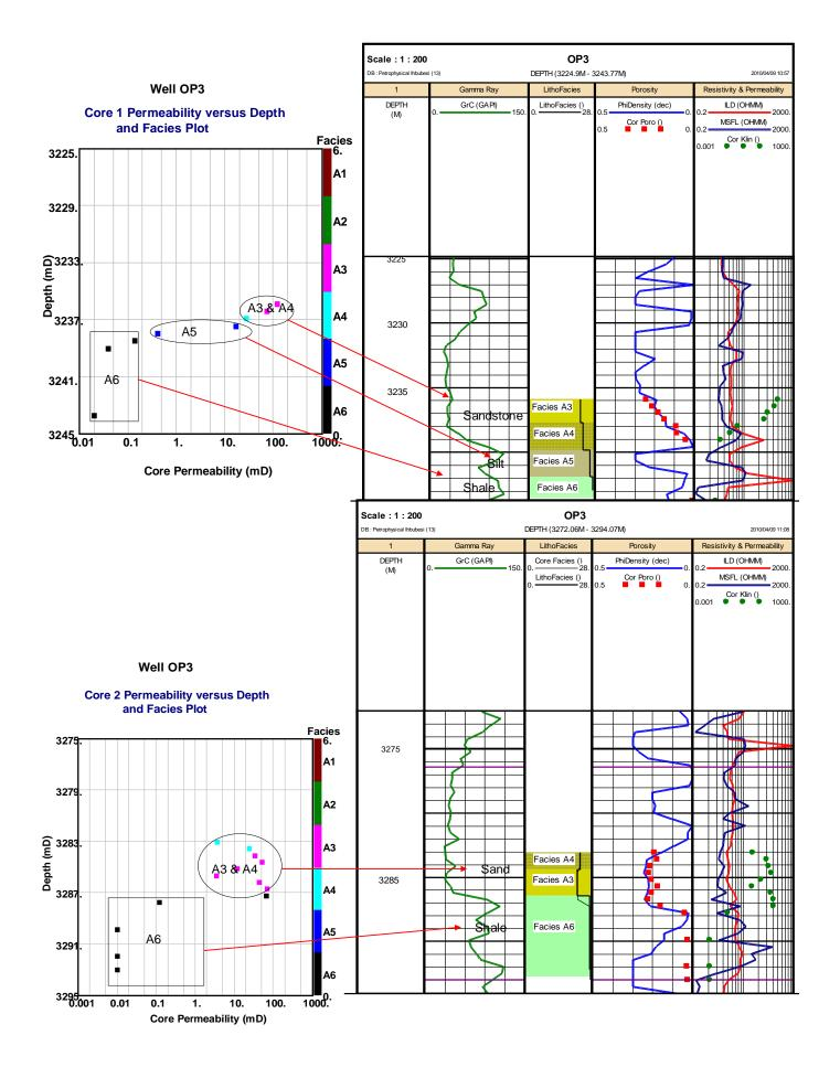
Figure 5.15a: Well OP3 depth-permeability plot.
