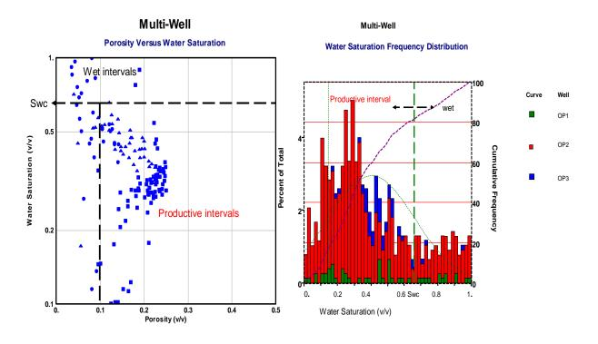
Figure 9.10: Multi-Well porosity vs water saturation and frequency distribution
