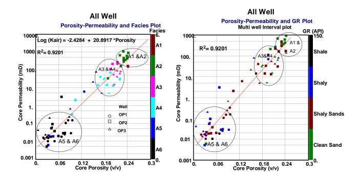
Figure 5.22: Porosity-permeability and facies distribution for wells
