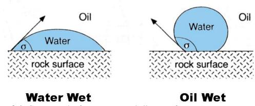
**Figure 3.6**: Contact angles for water-wet and oil-wet surfaces.
