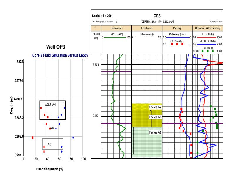
Figure 5.18b: Well OP3 core 2 fluid saturation versus depth plot
