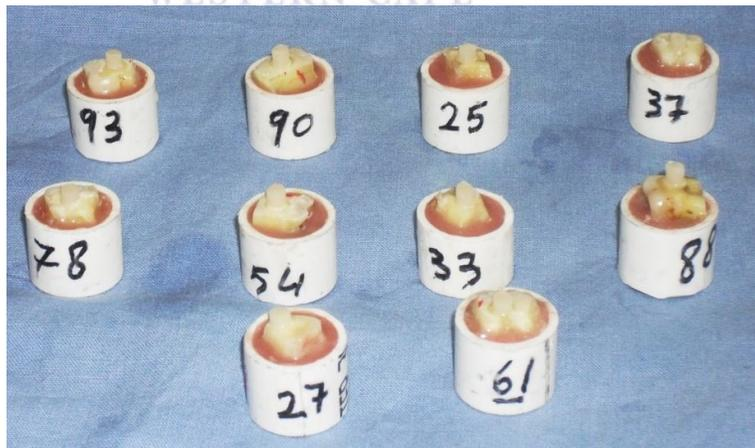
**Figure 4.10:** Composite mold bonded to prepared specimens after releasing from assembly.
