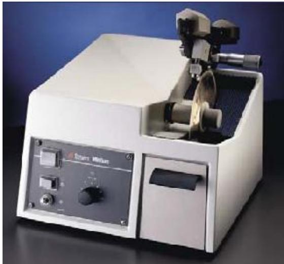
**Figure 4.5:** Water-cooled diamond disk-cutter (Minitom, Struers, Denmark).
