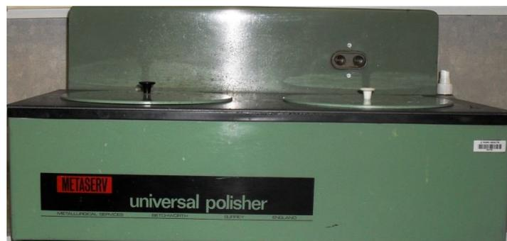
**Figure 4.7:** Universal polisher with 1200 grit silicon finishing paper.
