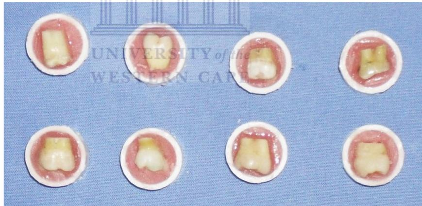
**Figure 4.4:** Embedded teeth in cold-cure acrylic resin.
