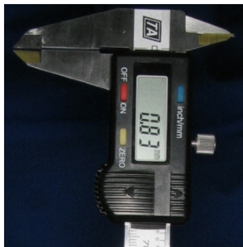
Figure 4.10: Electronic reading in 100 th of a mm
