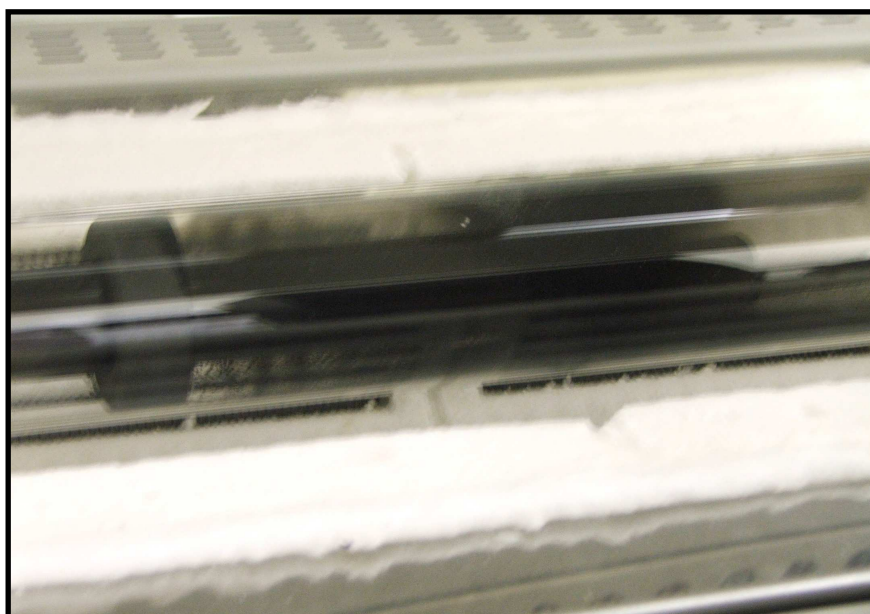
Figure 3.3: A Photograph of an open laser-ablation oven showing the target as well as the inner and outer quartz tubes.
