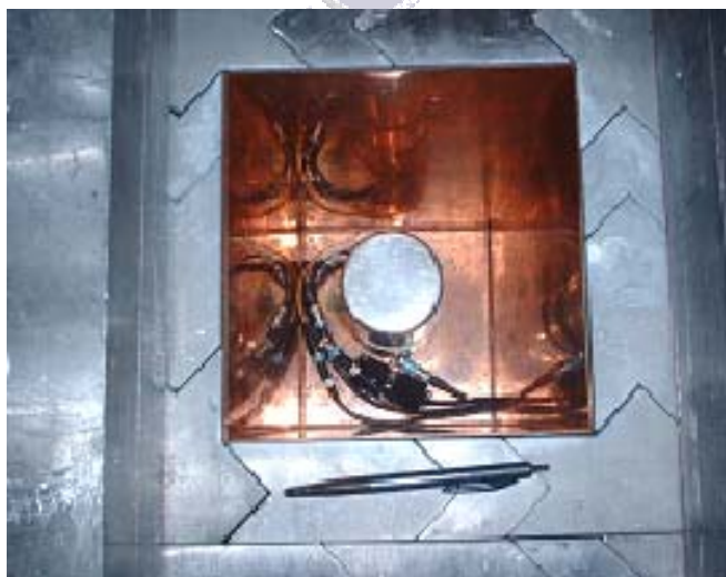
Figure 2.2: A photograph of the HPGe detector with accompanying lead castle used by the ERL.
