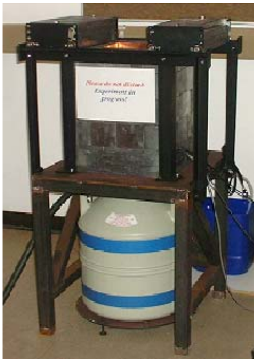
Figure 2.2: A photograph of the HPGe detector with accompanying lead castle used by the ERL.
