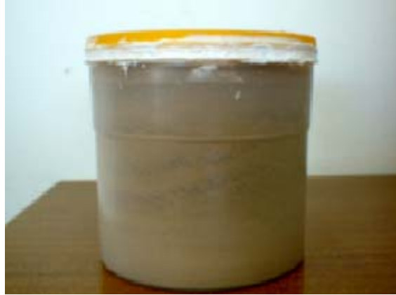
Figure 2.9: Sand sample sealed with copper disk and silicon in Marinelli beaker.
