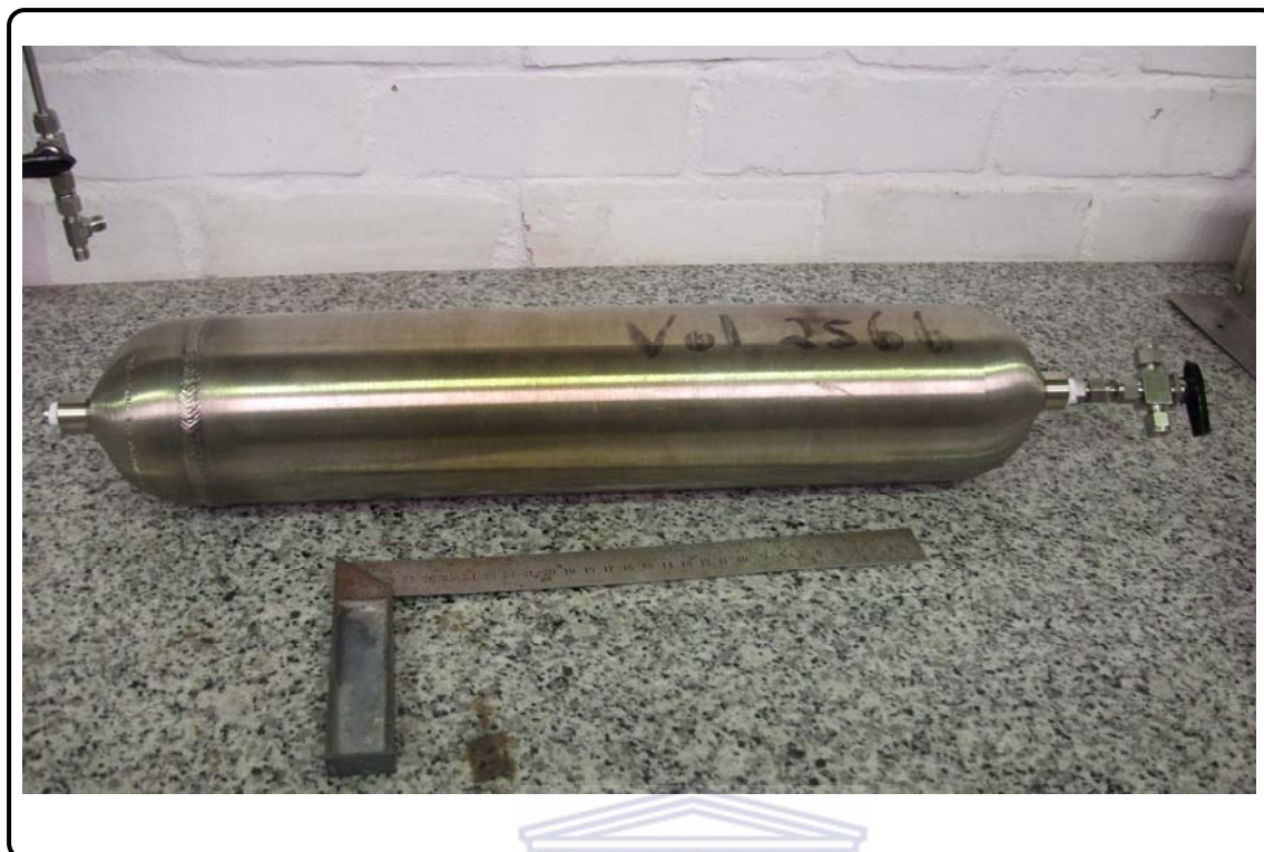
Figure 4.33: General view of the assembled hydrogen storage unit
