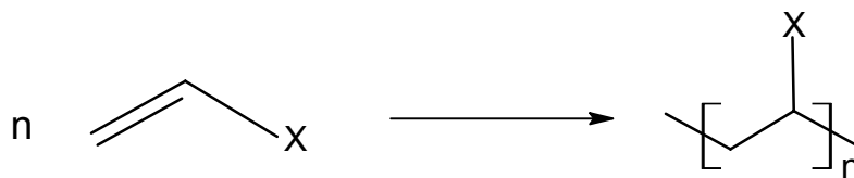
Figure 1.2: General addition polymerization
