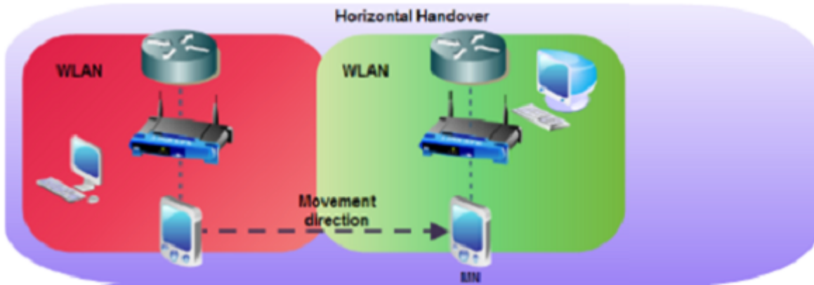
Figure 1.3: Horizontal handover - handover between homogeneous access technology. For example, the MN moves from WLAN subnet to the other WLAN subnet.
