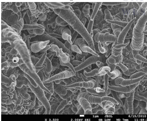
Figure 4.4: SEM images: (G) electrochemically polymerized G2PPI-co-PPy ( \times 3500 ), (H) electrochemically polymerized G2PPI-co-PPy ( \times 10,000 ), (I) electrochemically polymerized G3PPI-co-PPy ( \times 2000 ), (J) electrochemically polymerized G3PPI-co-PPy ( \times 10,000 ), (K) electrochemically polymerized G4PPI-co-PPy ( \times 3500 ), and (L) electrochemically polymerized G4PPI-co-PPy ( \times 3500 ).
