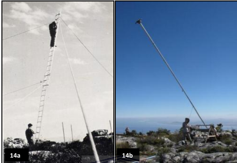
Figure 14a & b. The rope-suspended ladder photography system used by Coley during 1977 (Figure 14a) and the boom system used in 2010 (Figure 14b).
