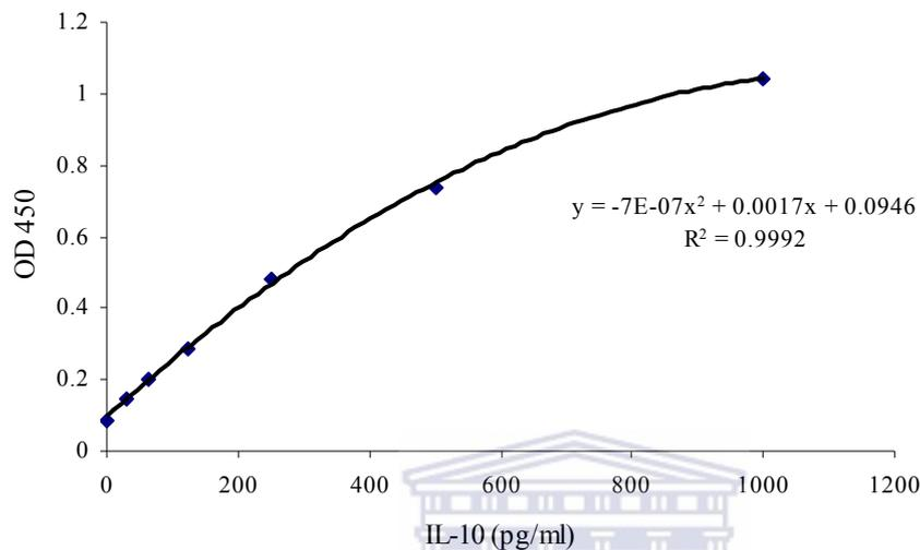
**Figure 4b:** Standard curve for IL-10. The kit standards were assayed by the DAS ELISA according to the manufacturer's instructions.
