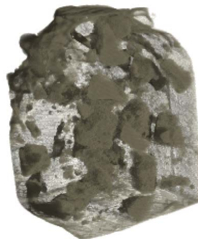
Figure 3-16: Software manipulated image of Ferro concrete sample-2 to only show aggregates embedded in cement paste within the concrete.
