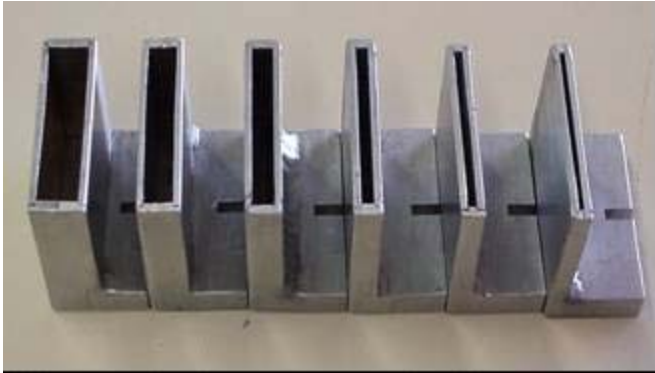
Figure 3-26: Aluminum sample holders of different thicknesses that can be filled with liquid.
