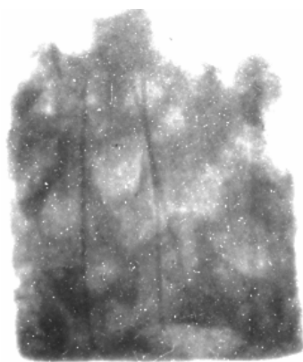
Figure 3-9: Neutron radiograph of the Ferro concrete sample at 0^{\circ} (starting position).
