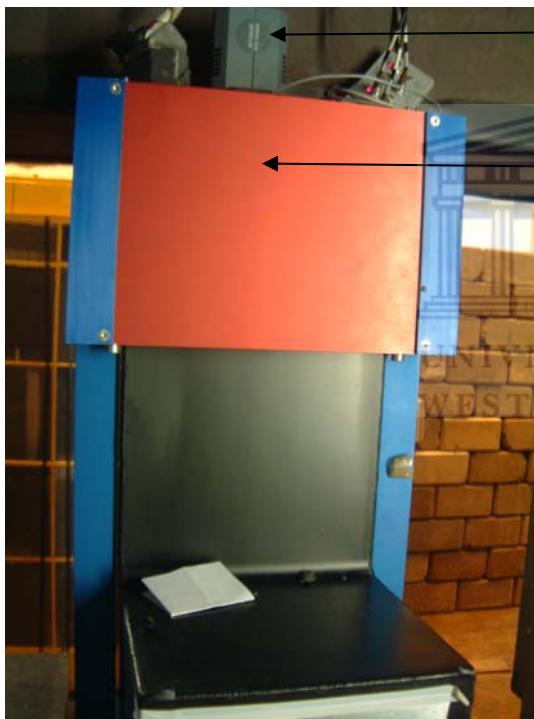
Figure 3-4: Photograph showing the upper part of the light-tight box. This houses the camera system on the top of the red component of the box.
