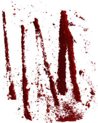
Figure 3-15: Software manipulated image of Ferro concrete sample-2 to only show the steel rods within the concrete.
