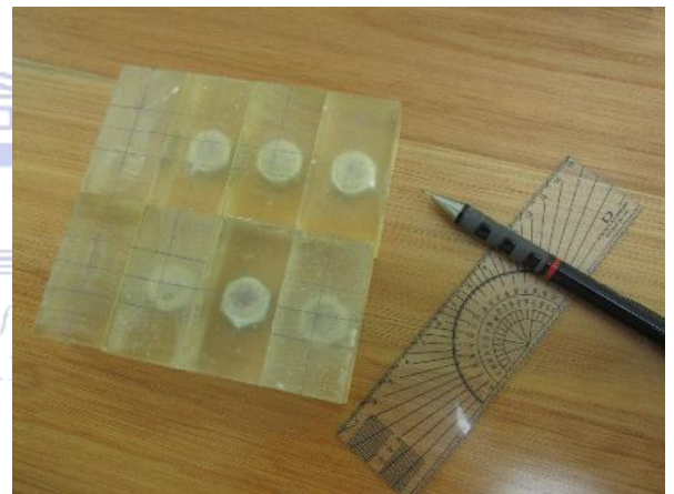
Figure 2: A measurement of 2 points 22 mm from each other and with equal distance from the edges of the block
