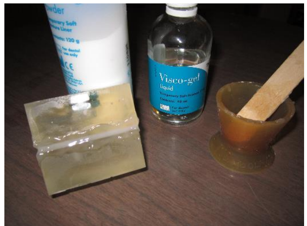
Figure 3: Application of Viscogel layer to the samples
