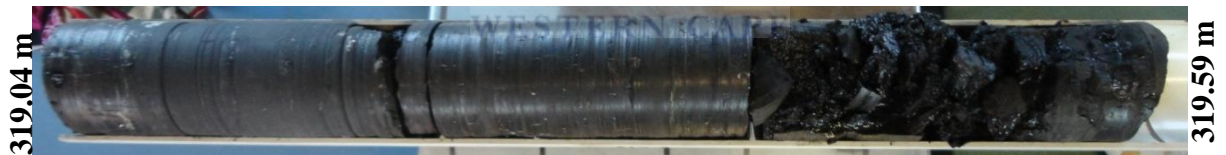
Figure 5.3.2: Sample D001 from borehole C6 (319.04 - 319.59 m depth), showing a zone of fracturing with calcite precipitation. This zone is interpreted as being the result of metasomatism caused by the movement of mobile fluids through the system. (Image supplied by Kubu Energy).
