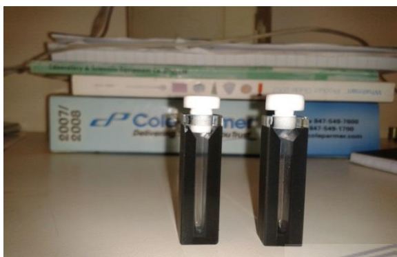
Figure 3-6: Cuvettes pieces used in UV-vis analysis of samples
