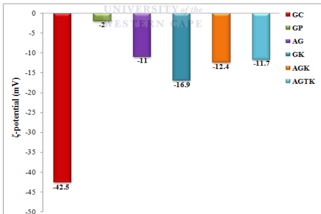
Figure 4.7: \zeta -potential of the AuNPs determined using Malvern Zetasizer as a measure of AuNP stability and charge. GC = citrate coated NPs, GP = PEGylated NPs, AG = targeted GP, GK = AuNPs with therapeutic peptide, AGK = has both targeting and therapeutic peptides, AGTK = has PTD, targeting and therapeutic peptides.
