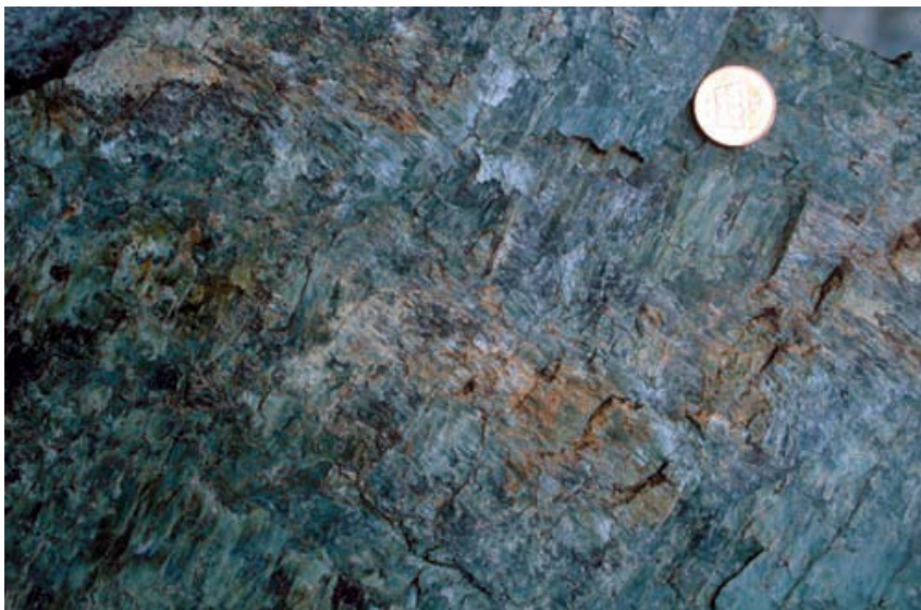
Figure 1.6. Two perpendicular sets of mineral lineations on a fault surface in serpentinite (Fossen, 2010)
