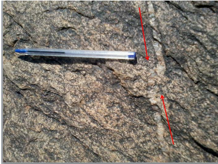
Figure 3.33 Quartz veins showing dextral rotation. Pen = 15 cm long.
