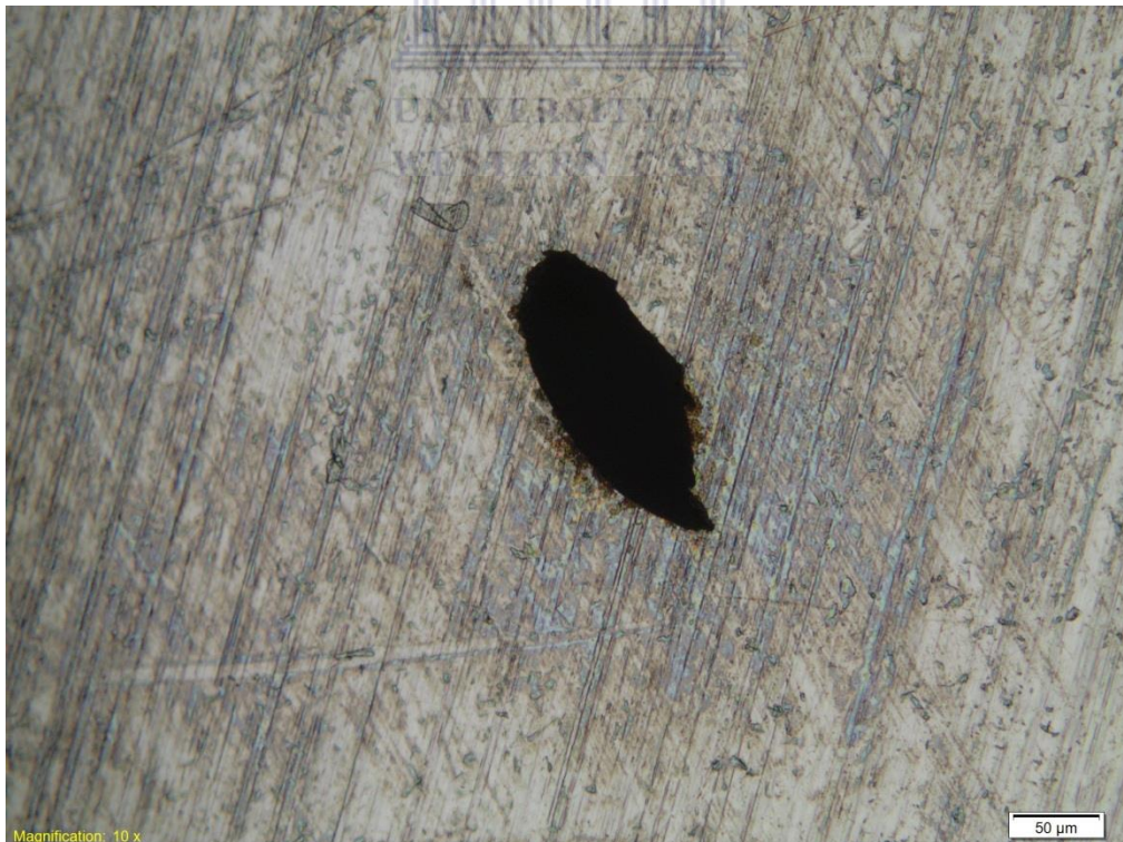
Figure 4.10: The entrance (a) and exit (b) holes drilled on a stainless steel 100 \mu\text{m} thick sheet using a Gaussian beam.
