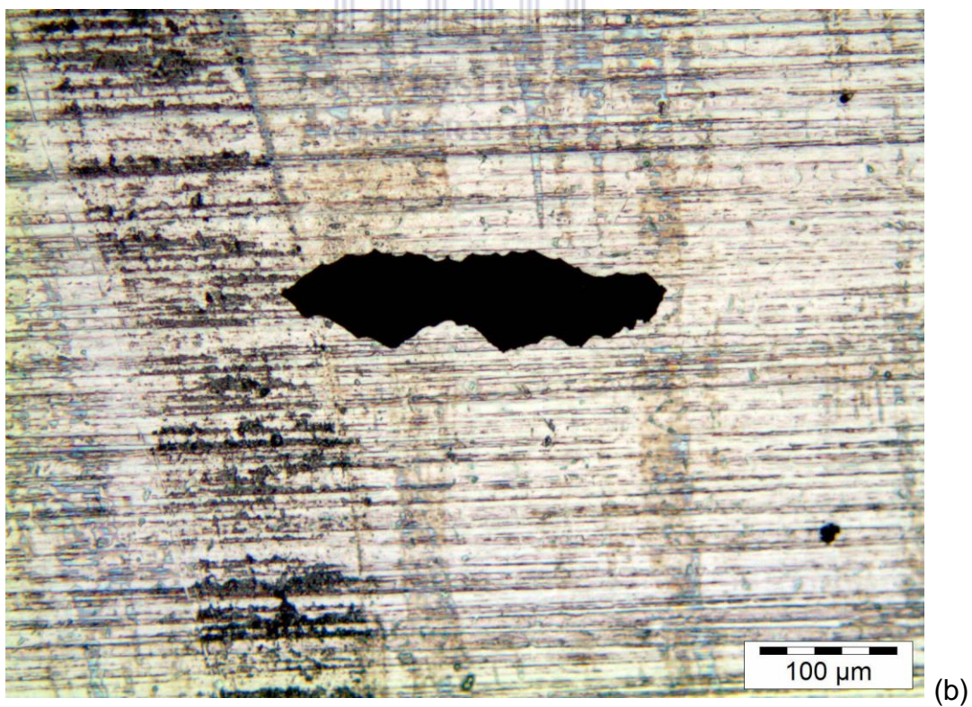
Figure 4.9: The entrance (a) and exit (b) holes drilled on a stainless steel 50 \mu\text{m} thick sheet using a Gaussian beam.
